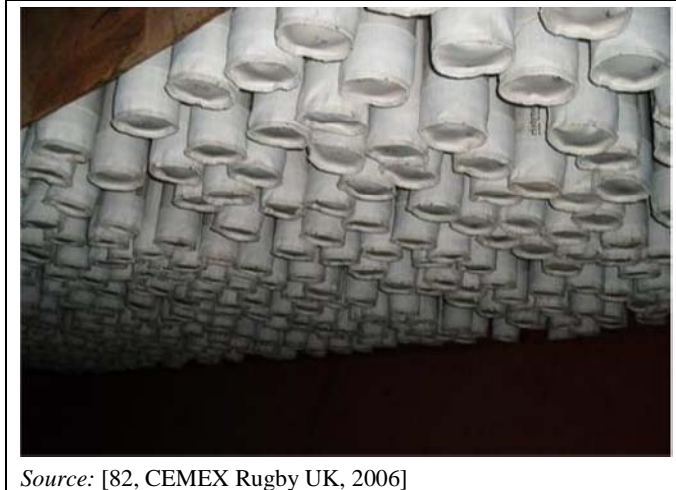
Figure 1.60: Example of a fabric filter and filter material used in a cement plant in the UK
