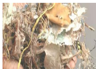
Figure 1.9: Specially prepared household waste used as fuel in cement kilns
