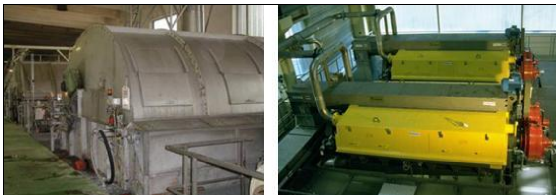
Figure 4.6: Example of a wash filter (left) and a wash press (right) in brown stock washing
