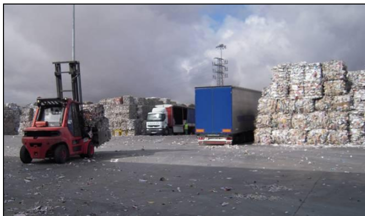
Figure 6.30: Outdoor storage of paper for recycling with concrete paving
