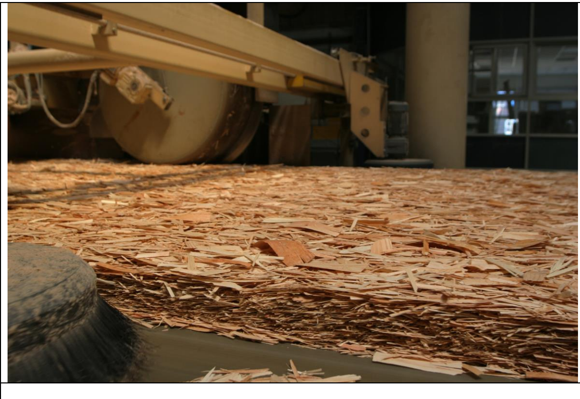
Figure 2.8: OSB mat after forming and trimming
