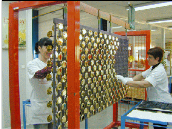
Figure 2.5: Jig or rack plating: unloading finished components Graingorge S.A., France and Agence de l'eau Seine-Normandie
