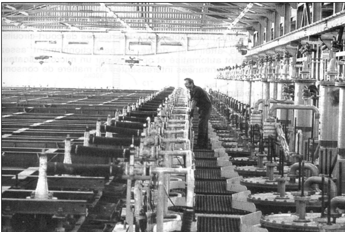
Figure 2.5: Mercury cells with vertical decomposer [Le Chlore, 1996]
