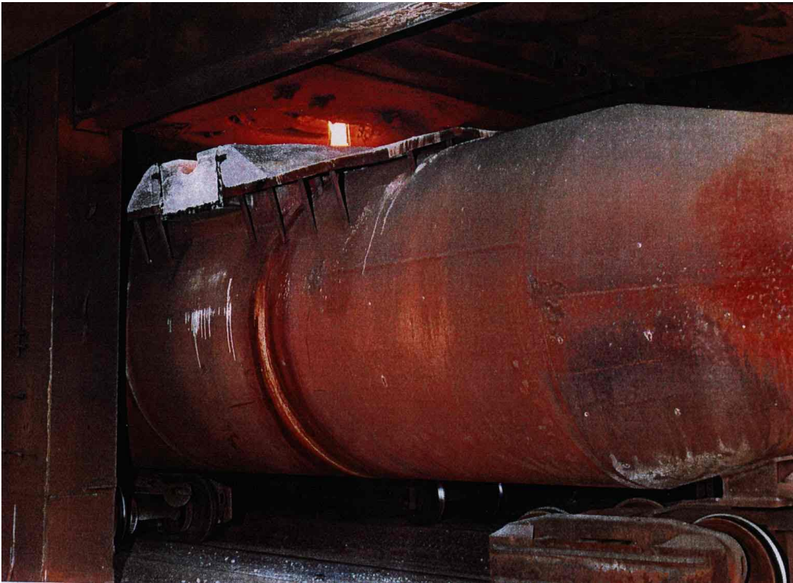
Figure 7.12 : Charging of hot metal into torpedo ladle with dust suppression with inert gas – [Haas, 1997].
