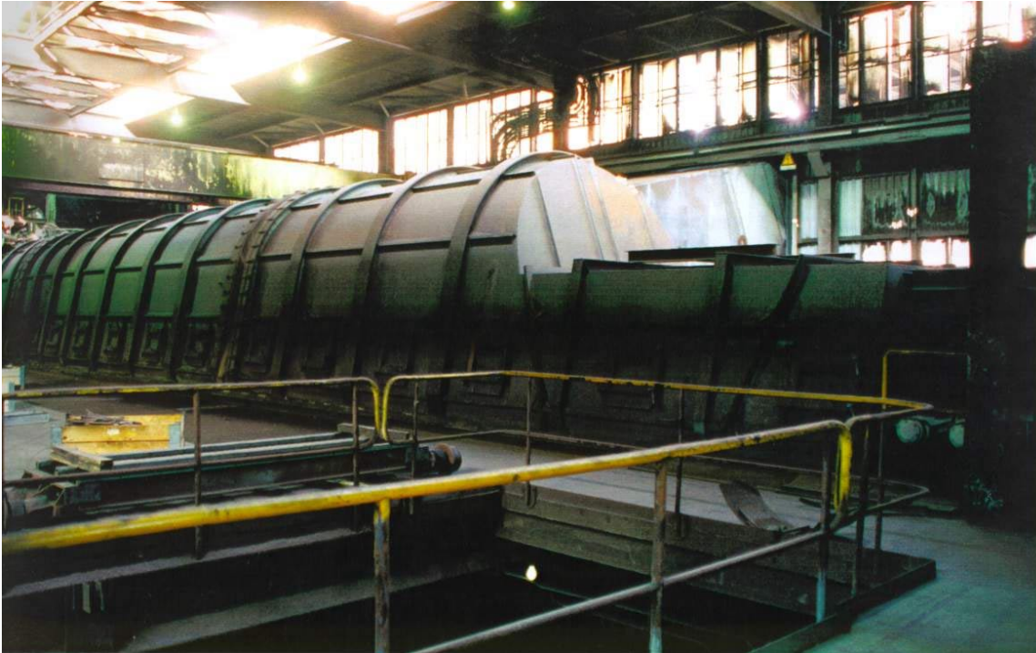
Figure 4.16 : Covered sinter strand according to the EOS process - [Panne, 1997]
