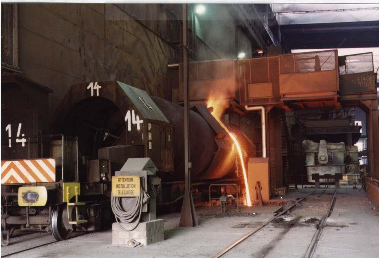
Figure 8.21: Reladling of hot metal from torpedo ladle to charging ladle with and without dust/fume suppression with inert gas (CO 2 ) [UNEP, 1997]
