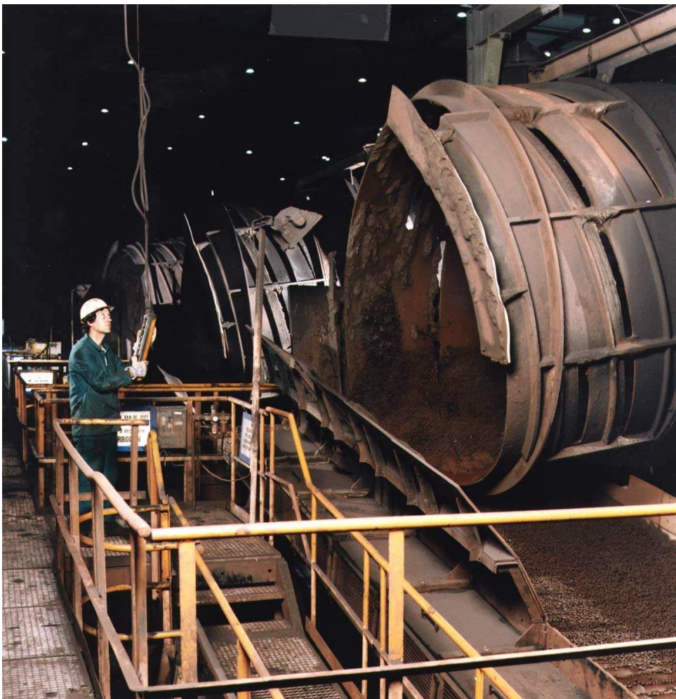
Figure 5.1 : Balling drum as part of a pelletisation plant
