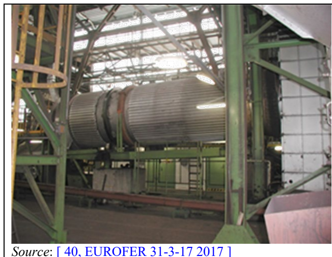
Figure 8.56: Picture of a rotary kiln for thermal treatment of oily mill scale at an ArcelorMittal integrated plant
