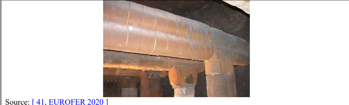
Figure 2.86: Double-pipes skid design for reheating furnaces
