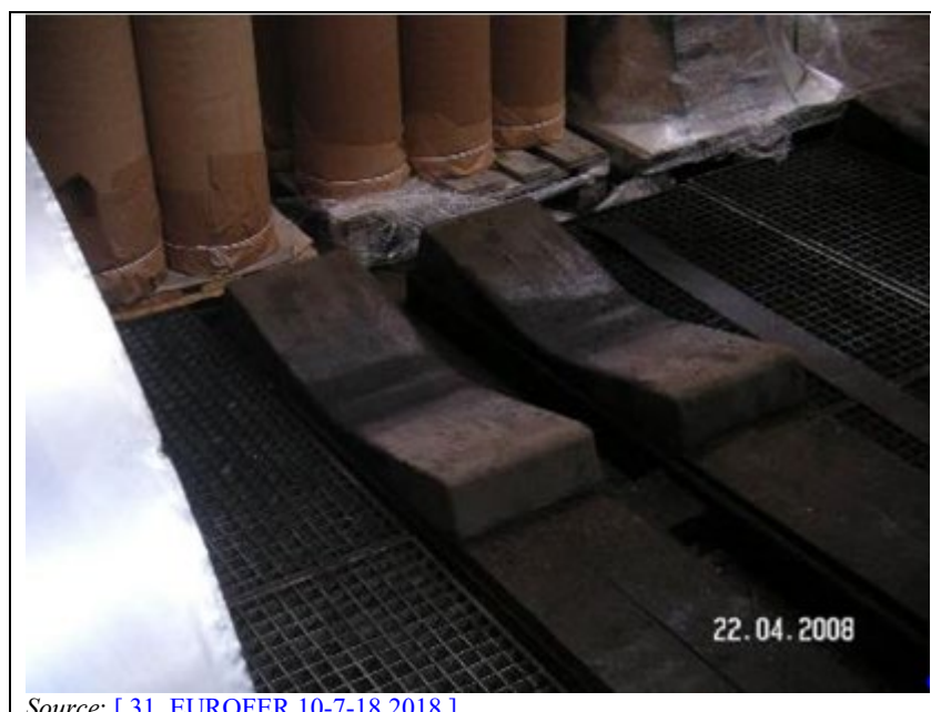
Figure 8.3: Coil support with oil drip trays
