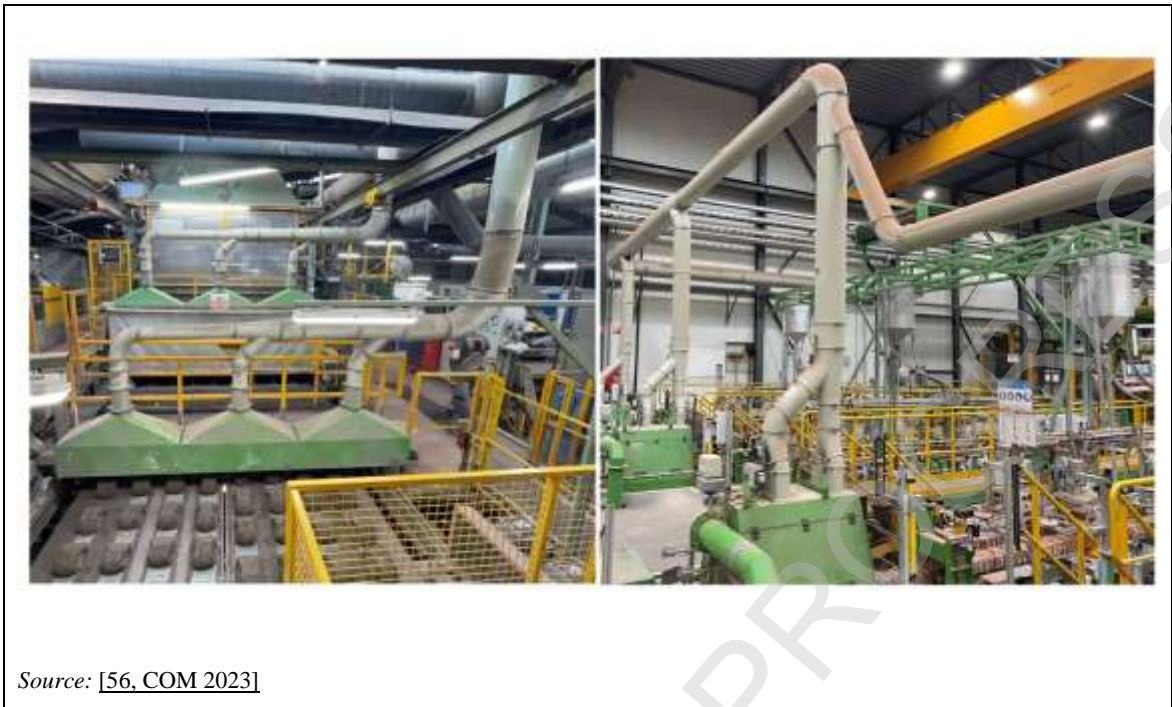
Figure 4-10: Channelling of dust emissions in facing brick manufacturing
