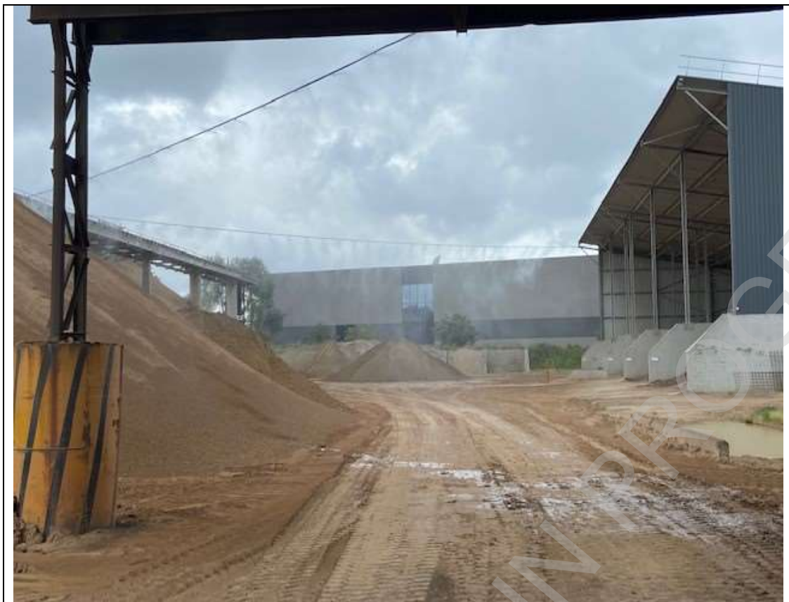
Figure 4-11: Example of a water sprays to reduce diffuse emissions in storage areas
