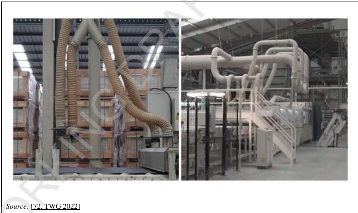
Figure 4-9: Channelling of dust emissions in wall and floor tiles manufacturing
