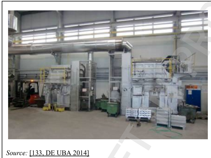
Figure 3.12: Exhaust systems of four furnaces connected with heat exchangers to transmit the heat of the hot gases from the melting process to the heating circuit
