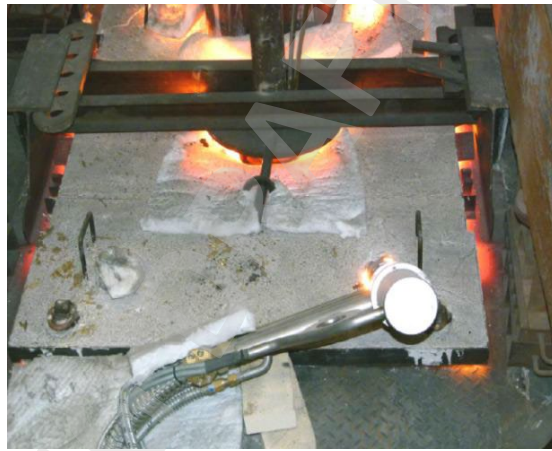
Figure 3.8: Oxy-fuel diffusion burner with cooling water, used here to heat the feeder during the casting of a ship propeller in a bronze alloy
