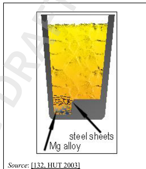
Figure 2.26: The sandwich method for nodularisation
