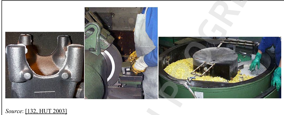
Figure 2.55: Burrs (L) and their removal using a grinding stone (C) and slide grinding (R)
