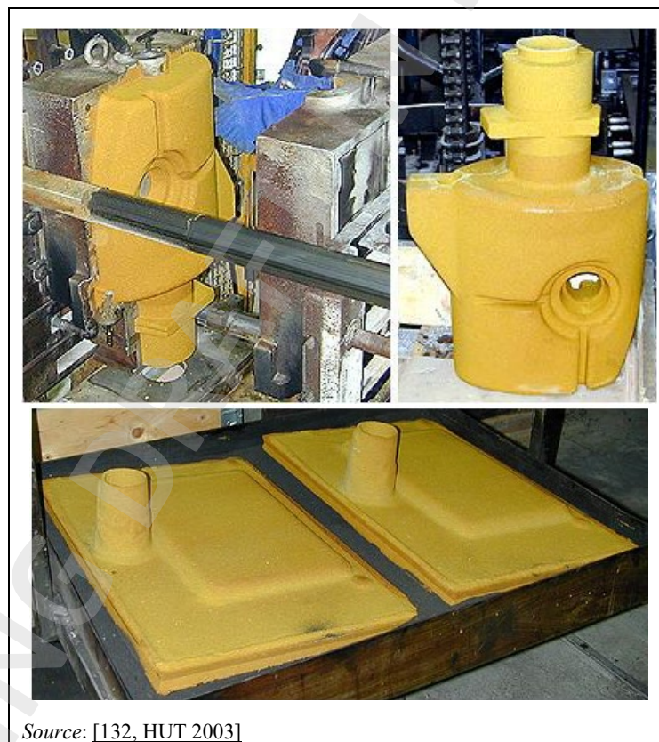
Figure 2.36: Croning cores (top) and moulds (bottom)
