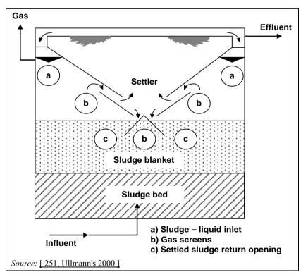
Figure 3.37: UASB process
