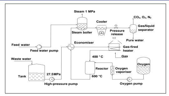
Figure 5.2: Simplified flow sheet of the SCWO process
