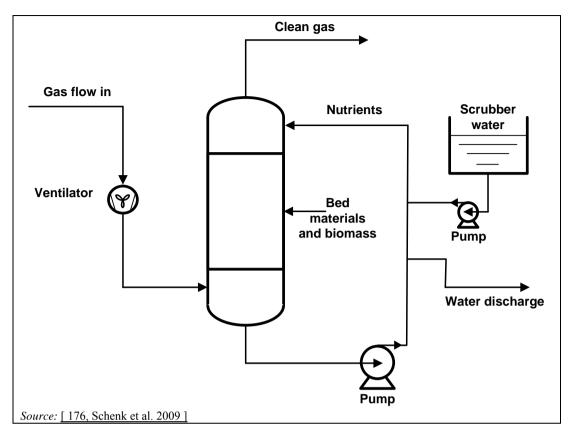
Figure 3.76: Typical biotrickling facility
