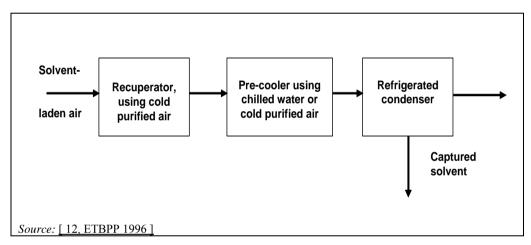
Figure 3.58: Two-stage condensation system
