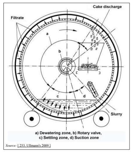
Figure 3.21: Rotary vacuum filter
