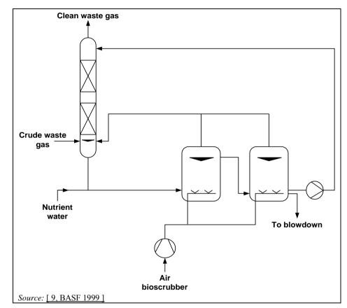
Figure 3.74: Typical bioscrubbing process
