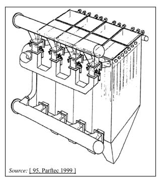
Figure 3.99: Metal mesh filter with recaking process
