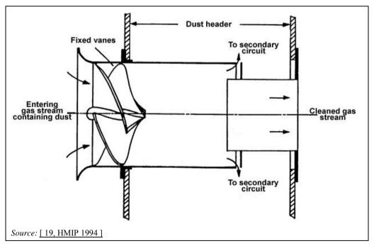
Figure 3.88: Straight-through cyclone
