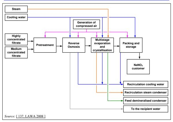
Figure 3.47: NITREA<sup>®</sup> treatment plant flow scheme
