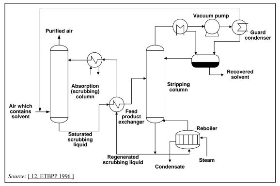
Figure 3.70: Typical absorption/desorption system
