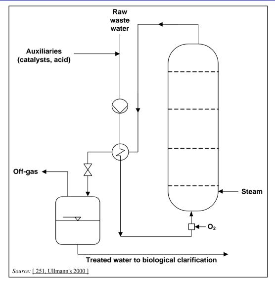
Figure 3.29: Flow diagram of a Loprox facility operated at 120–200 °C and 0.3–2.0 MPa with a retention time of < 3 h
