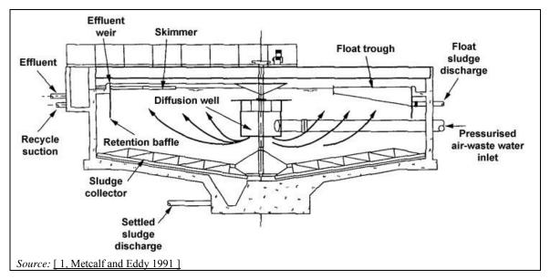
Figure 3.50: DAF thickener for waste activated sludge
