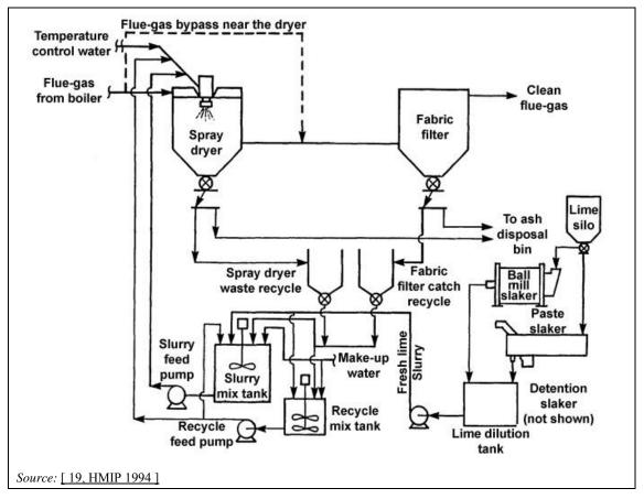
Figure 3.103: Spray or semi-dry sorbent injection system
