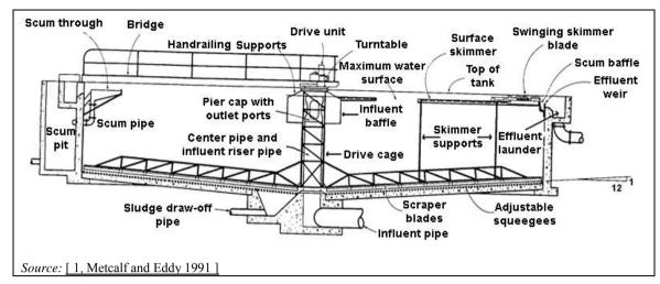
Figure 3.14: Circular sedimentation or settler tank
