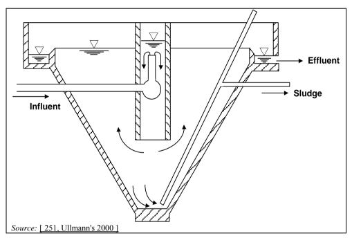
Figure 3.15: Hopper-bottom tank
