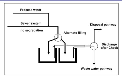
Figure 3.6: Self-contained buffer with alternative filling
