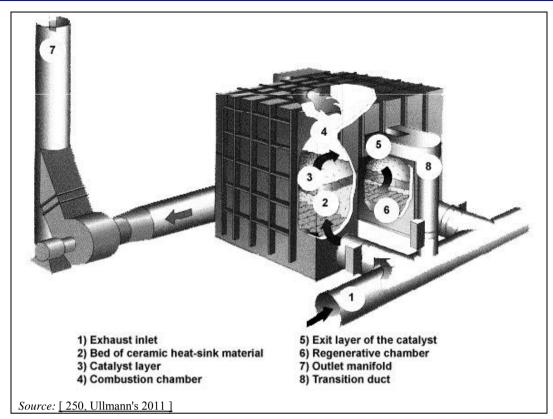
Figure 3.81: Regenerative catalytic oxidiser
