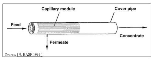
Figure 3.54: Typical membrane capillary module
