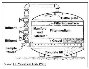
Figure 3.20: Pressure filter
