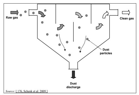
Figure 3.85: Settling chamber
