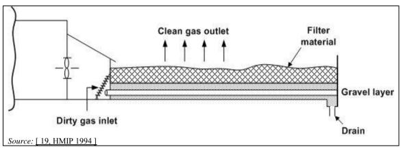
Figure 3.71: Biofilter construction
