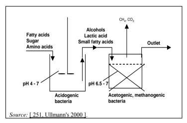
Figure 3.38: Two-stage anaerobic treatment process
