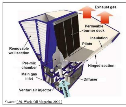
Figure 3.79: Principal components of the Clean Enclosed Burner<sup>®</sup>
