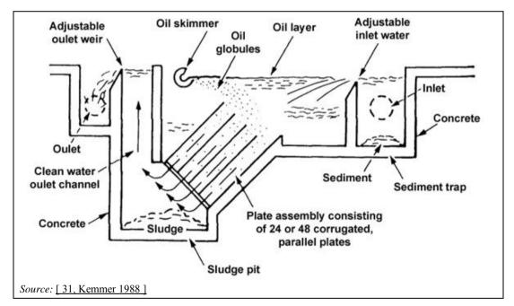
Figure 3.24: Corrugated plate interceptor (CPI)
