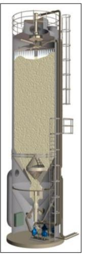
Figure 3.77: Moving-bed trickling filter
