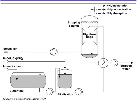
Figure 3.35: Air and steam stripping of ammonia
