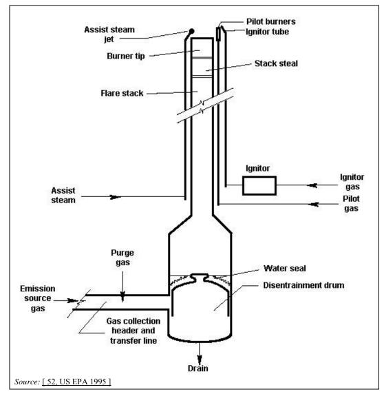
Figure 3.107: Typical elevated flare system
