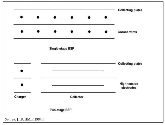
Figure 3.91: Single-stage and two-stage ESPs
