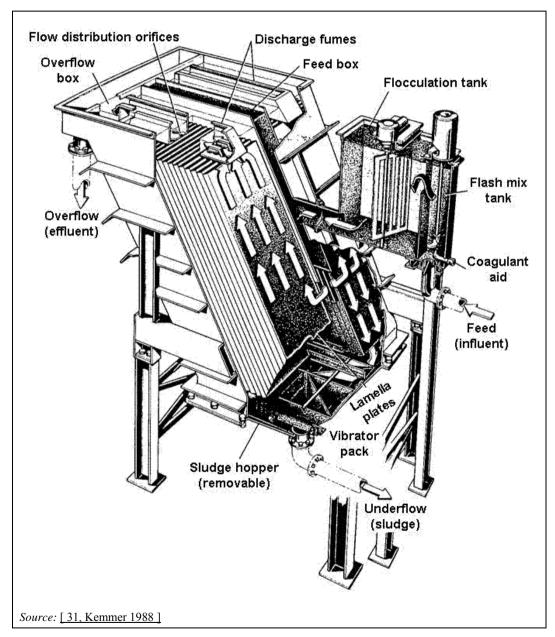
Figure 3.16: Lamina or tube settler
