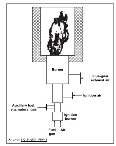
Figure 3.110: Muffle flare
