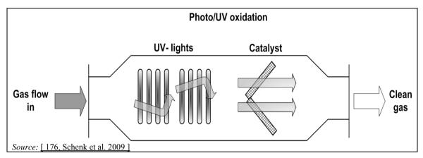
Figure 3.83: Photo/UV oxidation system
