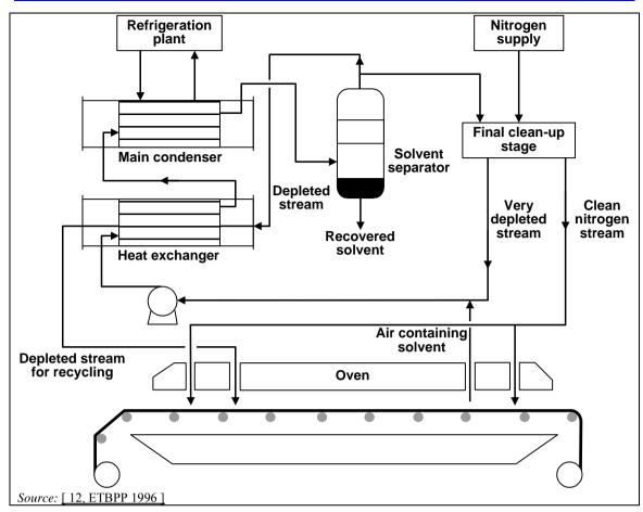
Figure 3.61: Typical closed-cycle inert gas condensation system
