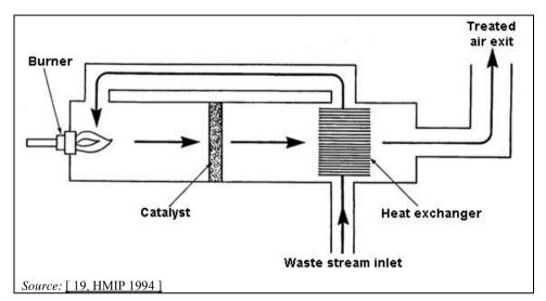
Figure 3.80: Principle of catalytic oxidation
