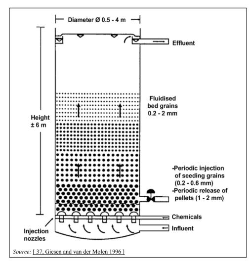
Figure 3.26: Principle of crystallisation process
