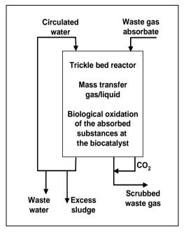
Figure 3.75: Flow sheet of the biotrickling process
