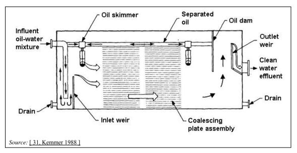
Figure 3.23: Parallel plate interceptor (PPI)
