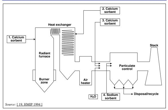
Figure 3.102: Dry sorbent injection for sulphur dioxide removal (injection positions)
