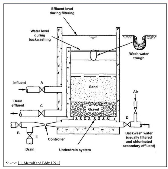
Figure 3.19: Conventional multi-media gravity-flow sand filter
