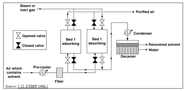
Figure 3.63: Example of a twin bed adsorption process
