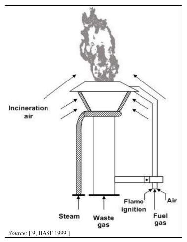
Figure 3.108: Injector rod flare
