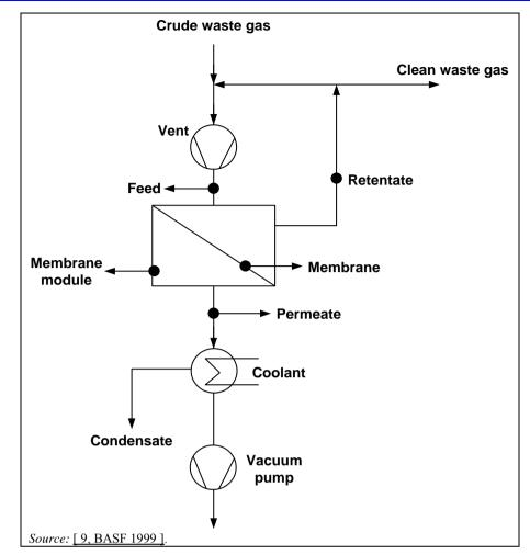
Figure 3.55: Common membrane separation system
