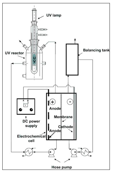
Figure 5.1: Example of a combined electrochemical oxidation process
