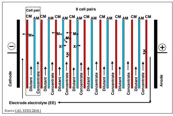
Figure 3.31: Electrodialysis
