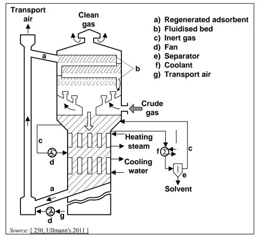
Figure 3.64: Fluidised-bed adsorption
