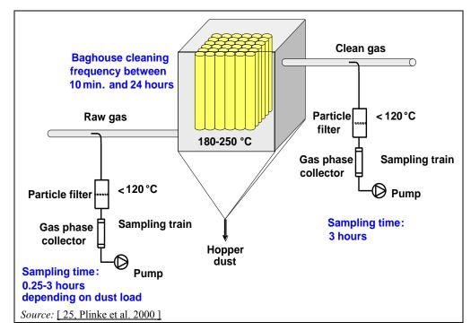
Figure 3.97: Catalytic filter baghouse, including sampling trains
