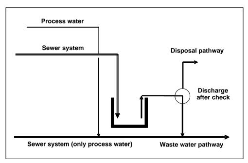
Figure 3.9: Leakage buffer system
