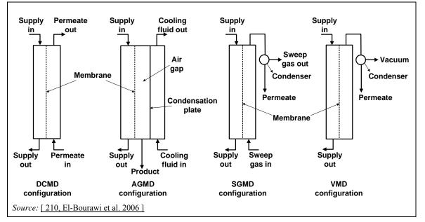
Figure 5.3: Different types of MD configurations
