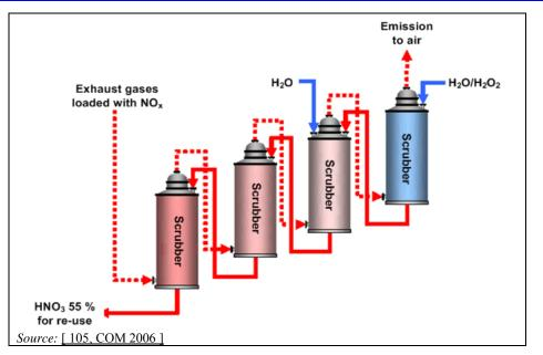
Figure 3.106: Recovery of NO<sub>X</sub> from waste gases with a scrubber cascade
