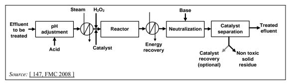
Figure 3.28: The wet oxidation with hydrogen peroxide technique
