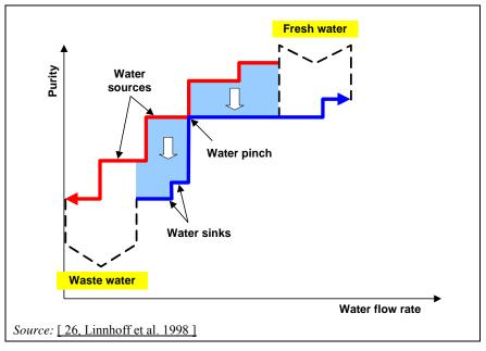
Figure 7.3: Pinch technology – analysis, source and sink curves
