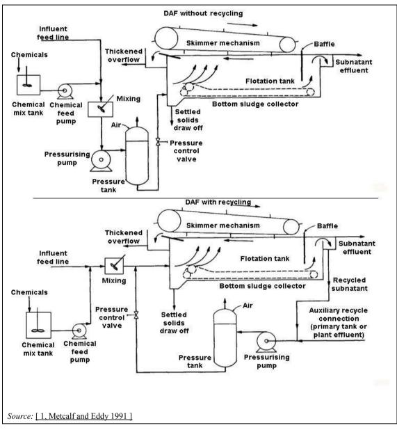
Figure 3.17: Dissolved air flotation with and without recycling
