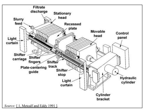
Figure 3.52: Fixed-volume recessed plate filter press
