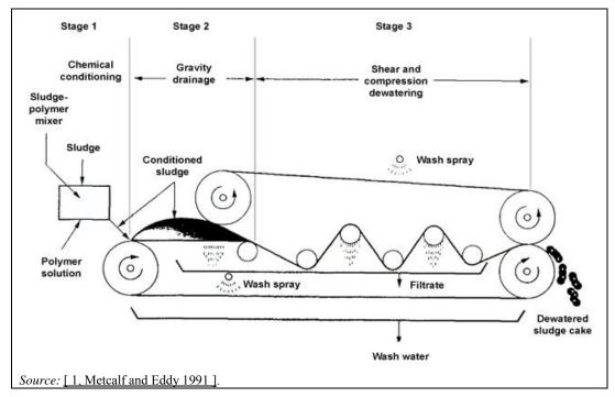
Figure 3.51: Belt filter press
