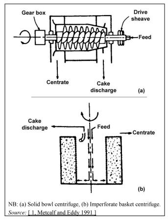
Figure 3.49: Centrifugal sludge thickener
