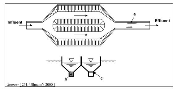
Figure 3.11: Channel-shaped horizontal-flow grit chamber
