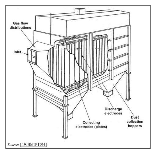
Figure 3.89: Wire plate ESP
