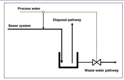
Figure 3.8: Connected buffer, continuously filled
