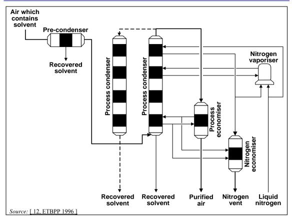
Figure 3.60: Cryogenic recovery system under inert atmosphere
