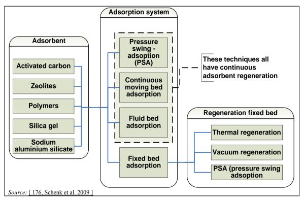
Figure 3.62: Overview of different adsorption systems, adsorbents and regeneration processes used
