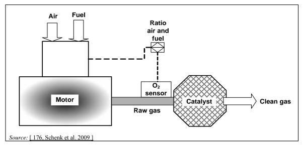
Figure 3.105: Non-selective catalytic reduction
