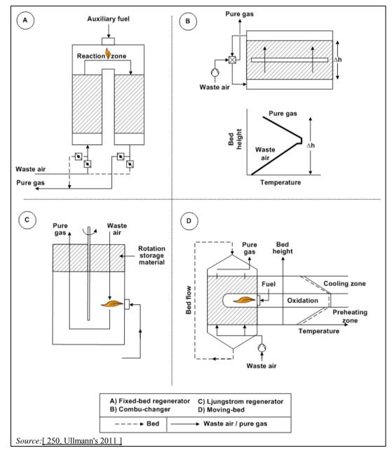
Figure 3.78: Schemes of various regenerative combustion systems
