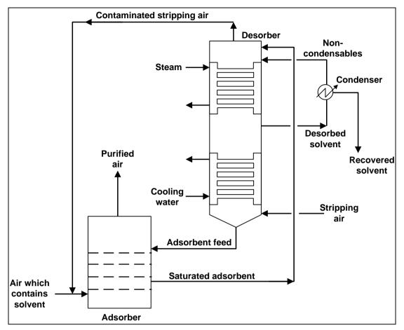
Figure 3.65: Continuous moving-bed adsorption and desorption
