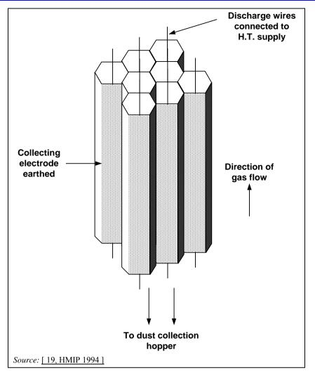
Figure 3.90: Dry wire pipe ESP
