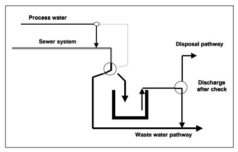
Figure 3.7: Connected buffer, discontinuously filled
