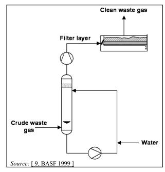
Figure 3.72: Typical biofilter process
