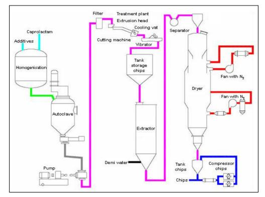
Figure 9.5 shows a simplified flow diagram of the process.
