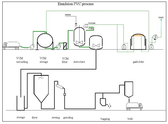
A flow diagram of an emulsion PVC process is shown in Figure 5.2.
