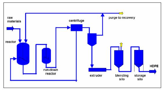
Figure 3.8: Flow diagram of an HDPE STR
