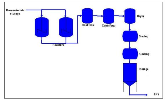
Figure 4.6: Flow diagram showing the EPS process
