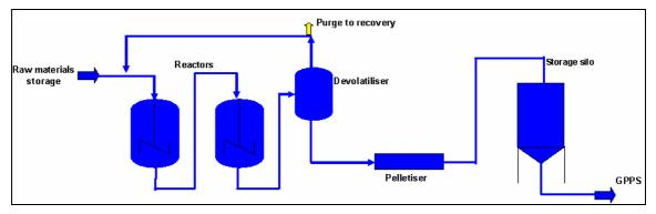
Figure 4.4: Flow diagram showing the GPPS process
