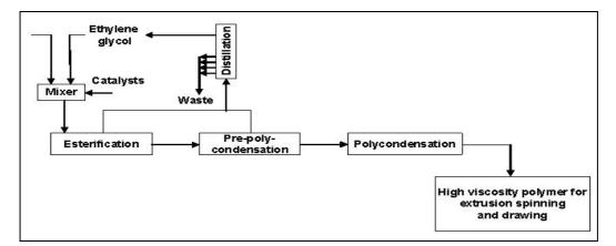
Figure 10.3: Flow chart of the PET TPA process
