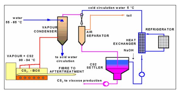
Figure 12.2: Schematic view of the condensation of CS<sub>2</sub> from viscose fibre production
