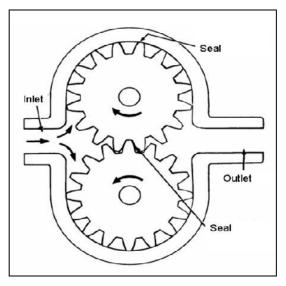
Figure 12.1: Schematic view of a gear pump
