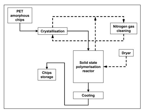
Figure 10.4: Flow diagram of continuous solid state polymerisation
