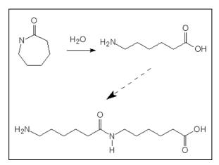
Figure 9.1: Basic reaction of AB type polyamides
