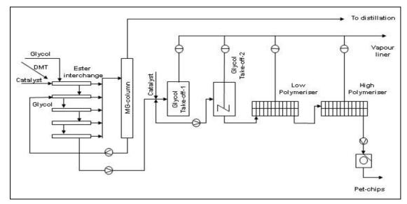
Figure 10.2: Flow chart of the PET DMT process
