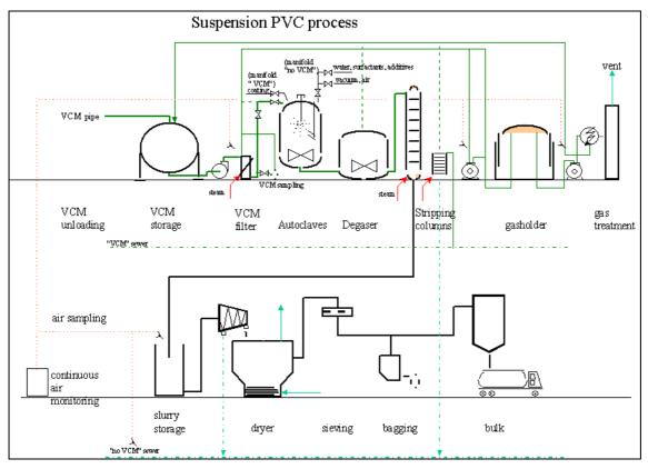
Figure 5.1: Flow diagram of an S-PVC process
