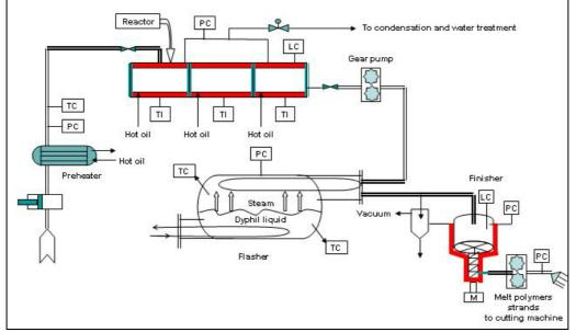
(LC = level control, PC = pressure control, TC = temperature control, TI = thermal insulation)
