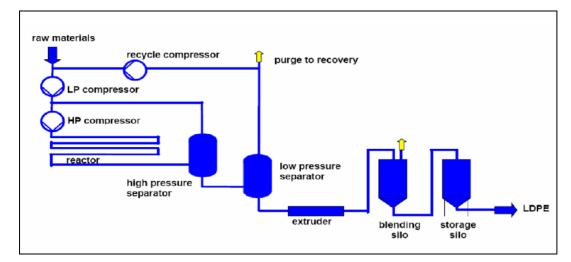
Figure 3.7: Flow diagram showing LDPE production
