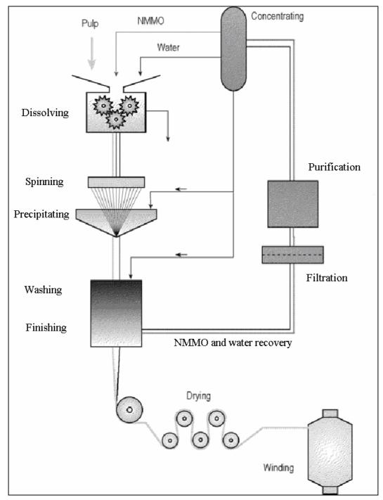
Figure 11.2 shows a simplified diagram of the Lyocell process.
