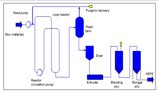
Figure 3.9: Flow diagram of an HDPE loop
