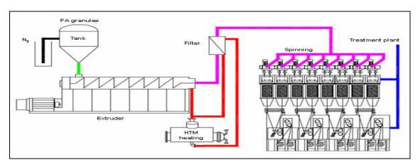
Figure 9.12: Flow chart of processing of BCF yarns
