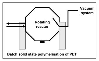
Figure 10.5: Schematic view of the batch solid state process
