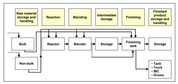
Figure 6.2 shows a schematic flow chart of the UP production process.
