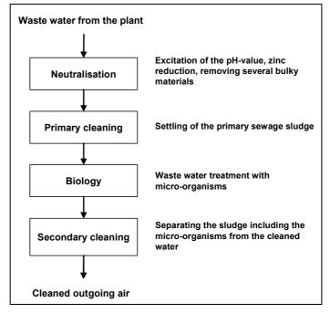
Figure 12.3: Schematic view of biological waste water treatment [43, Glanzstoff]
