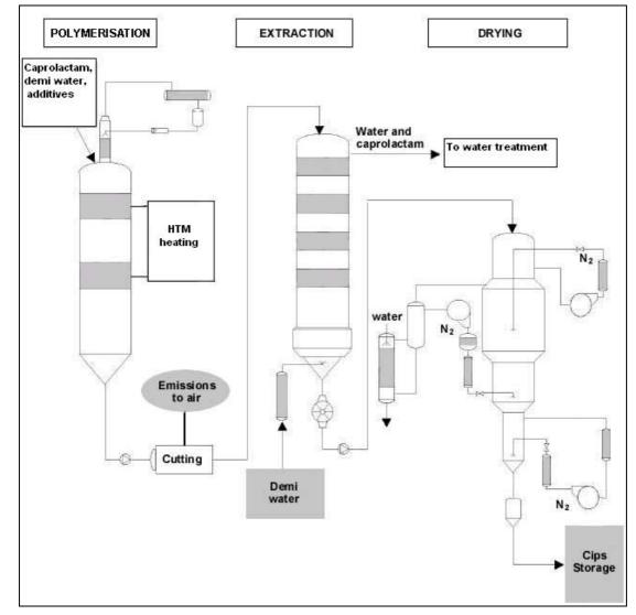
Figure 9.4 shows a simplified flow diagram of the process.
