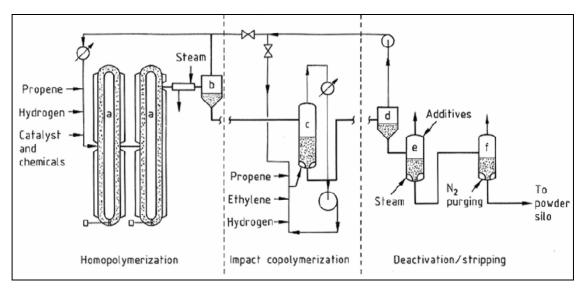
Figure 3.14: Flow diagram of the Spheripol polypropylene process [15, Ullmann, 2001]
