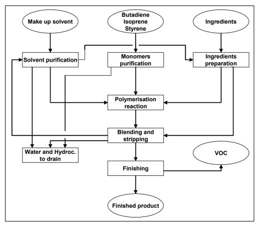
Figure 8.1. Principal flow scheme – solution polymerisation
