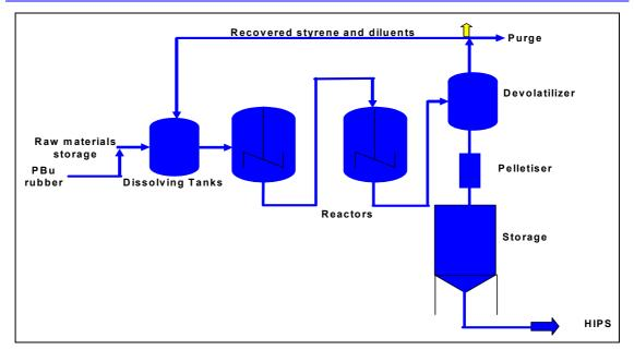
Figure 4.5: Flow diagram showing the HIPS process
