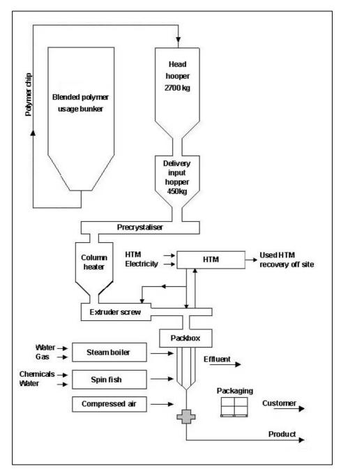
Figure 10.10: Flow chart of the production of filament yarns
