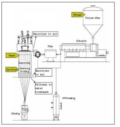
Figure 9.9: Flow diagram of the spinning process for textile yarns
