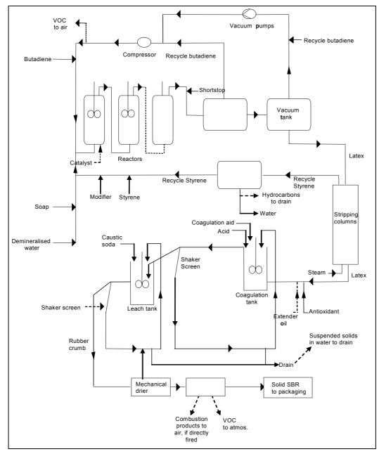
Figure 7.3: Flow diagram of the ESBR production process
