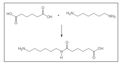
Figure 9.2: Basic reaction of AA-BB type polyamides
