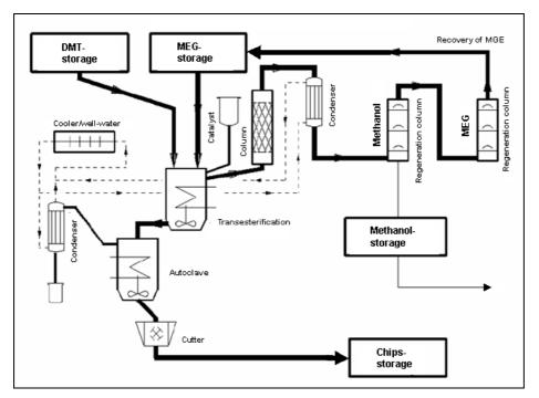
Figure 10.6: Flow diagram of the DMT-BPU process
