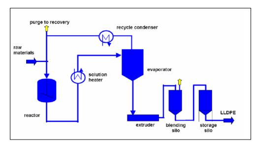
Figure 3.12: Flow diagram showing the LLDPE solution process
