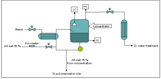
(*LC* = *level control*, *PC* = *pressure control*, *TC* = *temperature control*)
