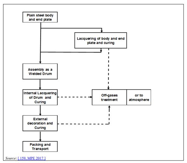
Figure 10.4: Production process of drums
