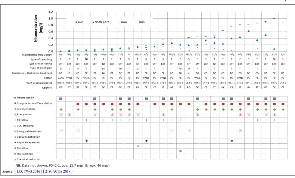
Figure 2.33: Ni concentration values for direct and indirect discharges of waste water from vehicle coating plants (data for 2015)
