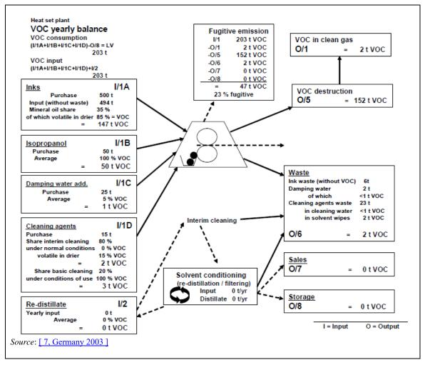
Figure 11.1: VOC balance of the virtual plant
