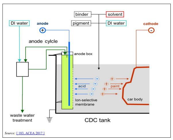
Figure 17.9: Electrocoating process
