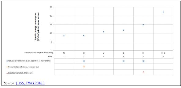
Figure 11.5: Specific energy consumption expressed in Wh per m<sup>2</sup> of printed paper surface (data for 2015)
