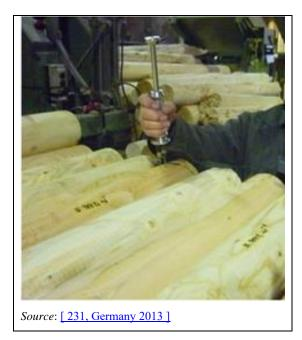
Figure 15.27: Manual wood moisture measurement
