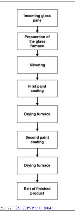
Figure 16.1: Flow chart of the manufacture of mirrors
