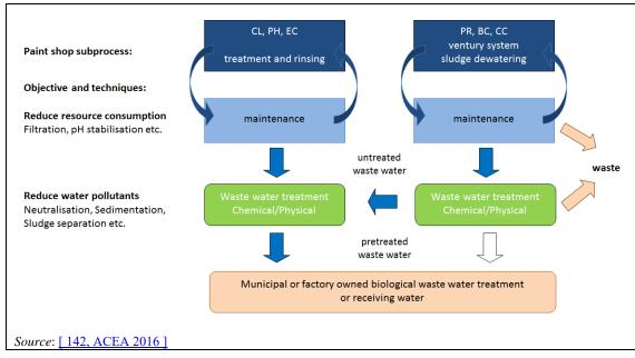
Figure 2.30: Typical technical configuration of waste water treatment in large paint shops
