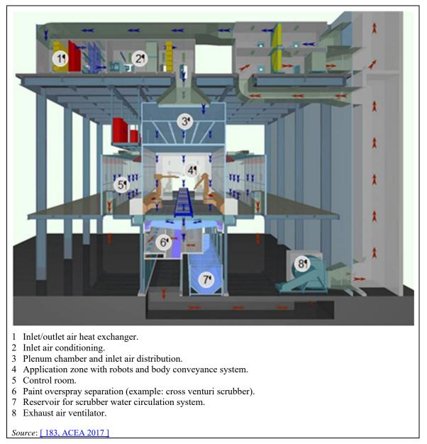
Figure 2.43: Structure and air conduction of a spray booth
