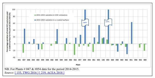
Figure 2.21: Percentage variation of total emissions of VOCs (g/m<sup>2</sup>) and total e-coated surface for 2013-2015
