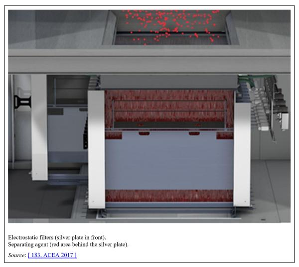
Figure 2.46: Detail of electrostatic filters and application of separating agent
