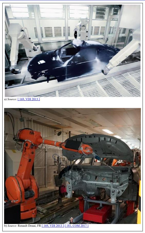
Figure 2.41: a) Automated paint application using robots and b) automated sealant application using robots
