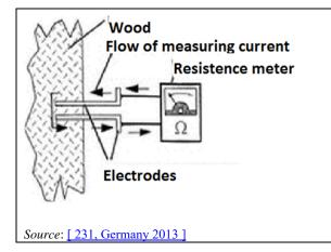
Figure 15.26: Basic principle of electric resistance wood moisture measurement
