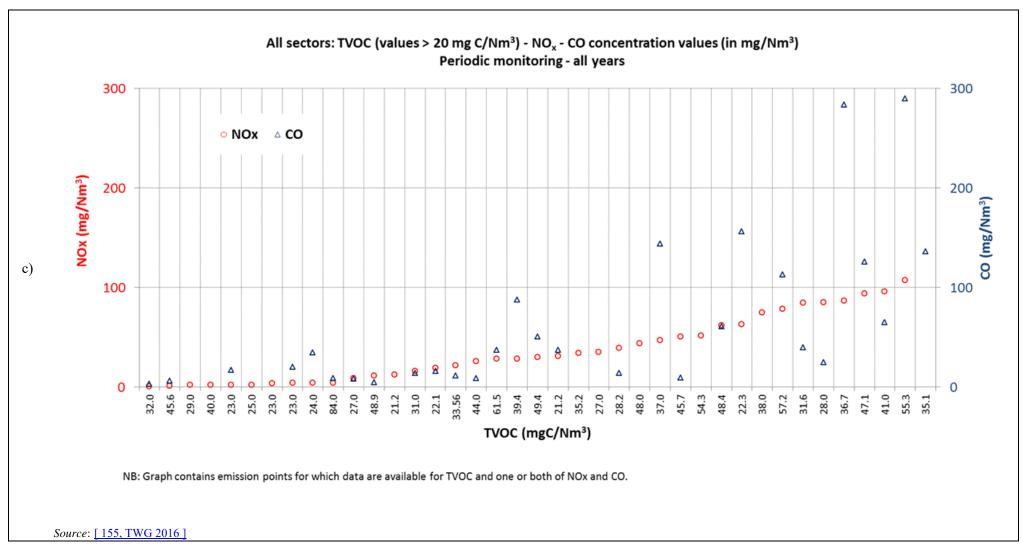
Figure 17.18: Reported emission levels of TVOC, NO<sub>X</sub> and CO from plants from all STS sectors where thermal treatment is applied
