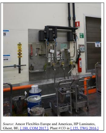
Figure 17.4: Automatic mixing system in flexography plant
