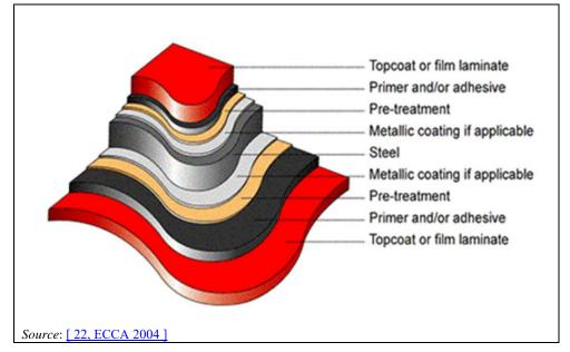
Figure 6.2: Typical layers of a coated steel product
