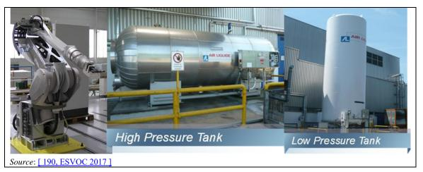
Figure 17.14: (a) Applicator robot, (b) High-pressure CO<sub>2</sub> tank, (c) Low-pressure CO<sub>2</sub> tank
