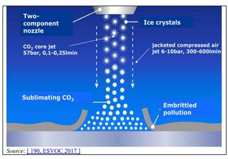
Figure 17.13:Liquid CO2 discharge
