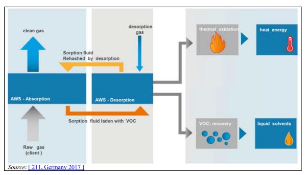
Figure 17.25: Scheme of the absorption off-gas treatment system
