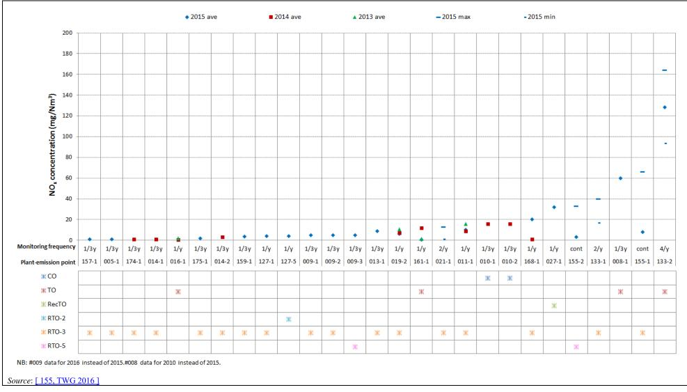
Figure 12.8: NO<sub>x</sub> emissions in waste gases for the period 2013-2015
