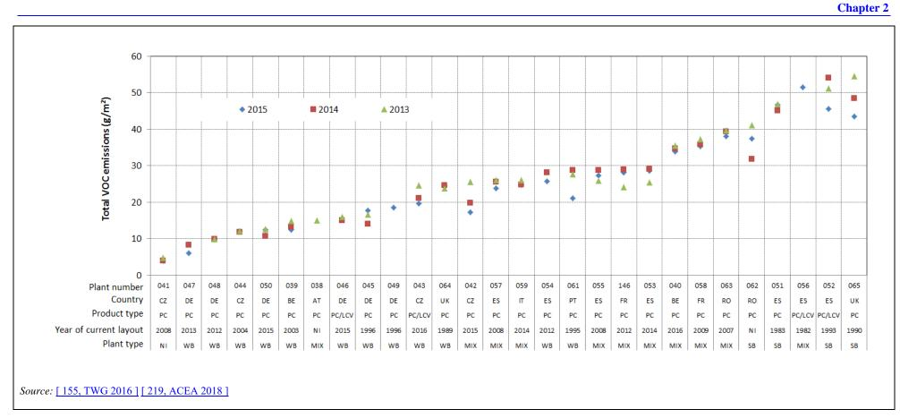
Figure 2.20: Total emissions of VOCs (g/m<sup>2</sup>) from the coating of passenger cars for the period 2013-2015
