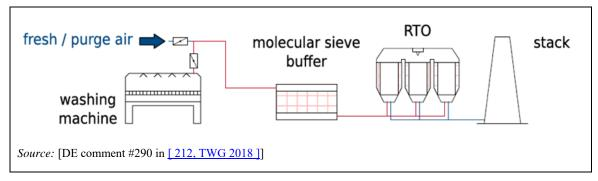
Figure 17.19: Scheme of the molecular-sieve-buffer-assisted exhaust treatment system
