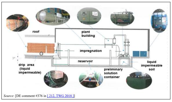
Figure 15.9: Example of a water-based pressure treatment plant with an open mixing/storage tank
