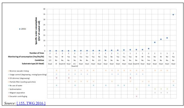
Figure 6.3: Specific water consumption expressed in 1 per m<sup>2</sup> of coated coil product (data for 2015)
