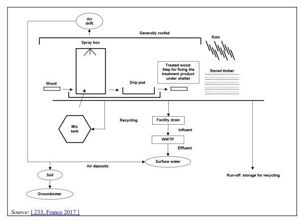
Figure 15.6: Flow diagram for spraying / spray tunnel process
