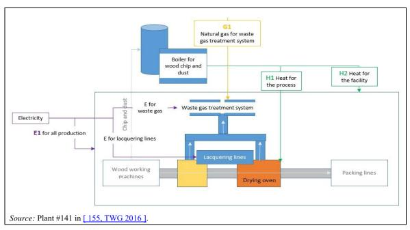
**Figure 14.2:** Schematic diagram of the energy inputs
