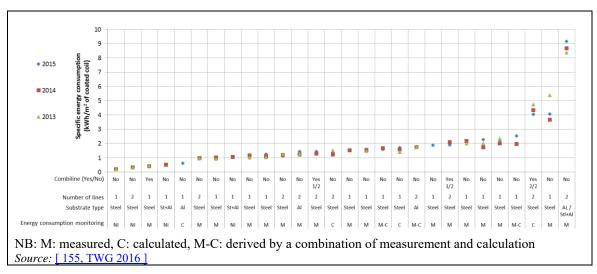
Figure 6.4: Specific energy consumption expressed in kWh per m<sup>2</sup> of coated coil product for period 2013-2015
