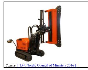
Figure 4.3: Box around the spear head in some more advanced robot models
