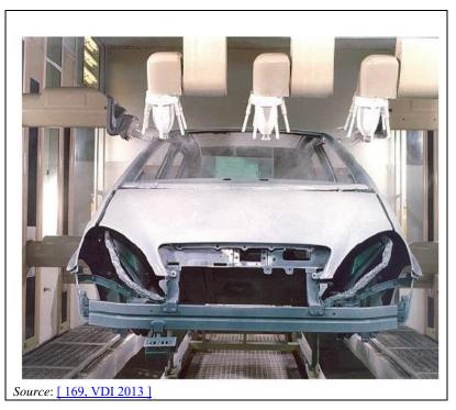
Figure 2.40: Automated paint application using painting machines
