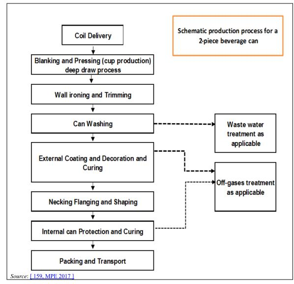
Figure 10.1: Production process for beverage cans
