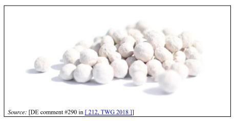
Figure 17.21: Pelletised natural molecular sieve (zeolite)
