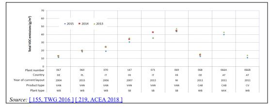
Figure 2.22: Total emissions of VOCs (g/m<sup>2</sup>) from the coating of vans, trucks and truck cabins for the period 2013-2015
