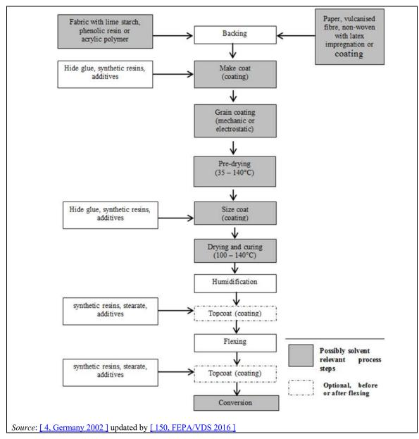
Figure 16.3: Schematic process flow for coated abrasives
