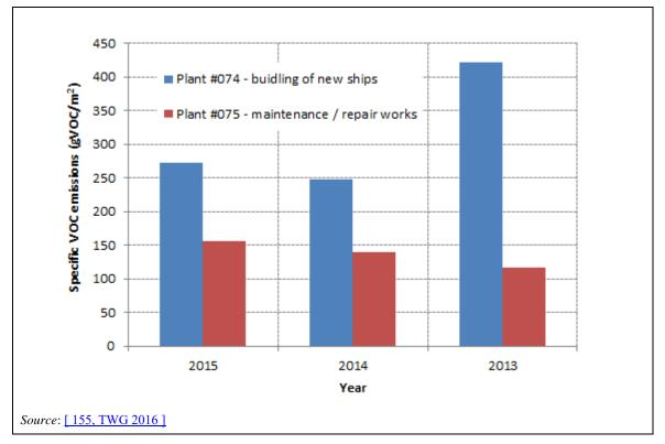
Figure 4.1: Total emissions of VOCs expressed in g VOCs per m<sup>2</sup> of coated surface for two plants for the period 2013-2015
