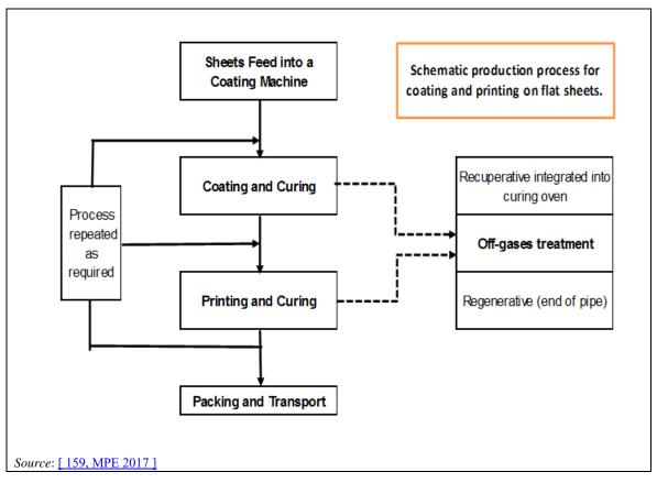
Figure 10.5: Production process for flat metallic sheet
