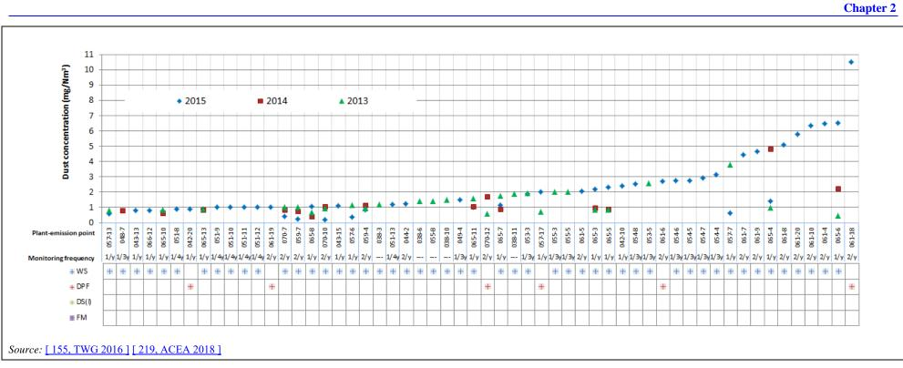
Figure 2.24: Dust emissions in waste gases (periodic monitoring) - Average values for the period 2013-2015 (2/2)
