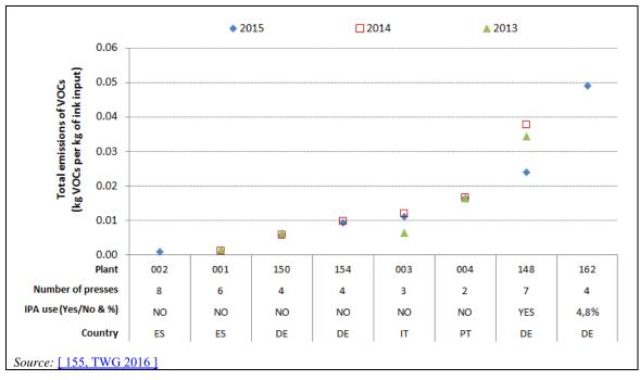
Figure 11.6: Total emissions of VOCs expressed in kg VOCs per kg of ink input for the period 2013-2015
