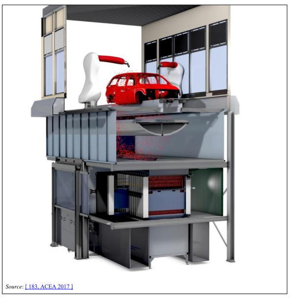
Figure 2.45: Rinsed electrofilter system
