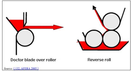
Figure 7.2: Different types of adhesive application units
