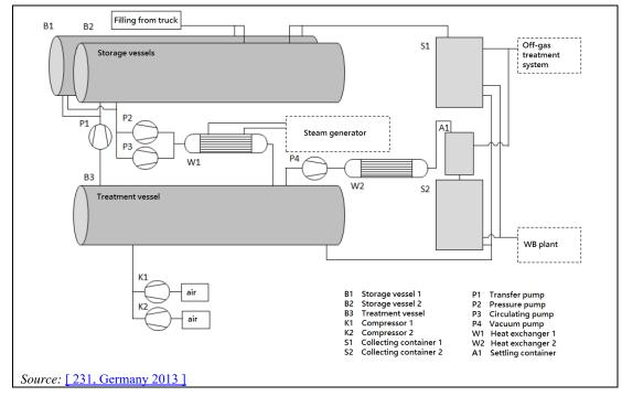
Figure 15.30: Schematic of Plant DE-1
