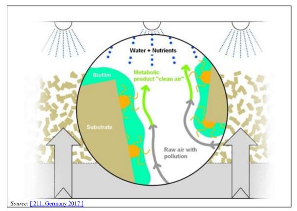
Figure 17.31: Reactor for biological off-gas treatment
