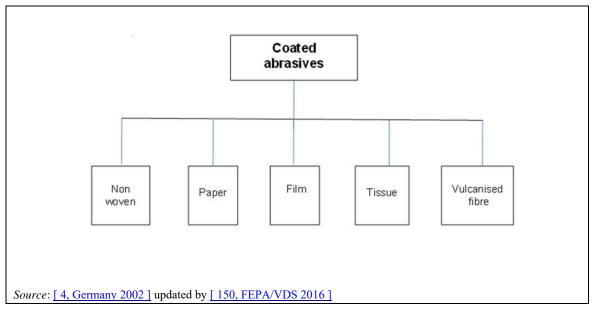
Figure 16.2: Overview of different types of coated abrasives
