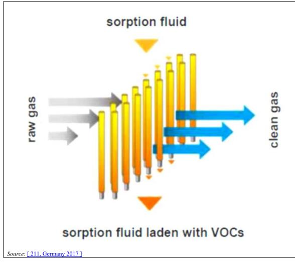
Figure 17.26: Cross-counter flow in the absorption unit
