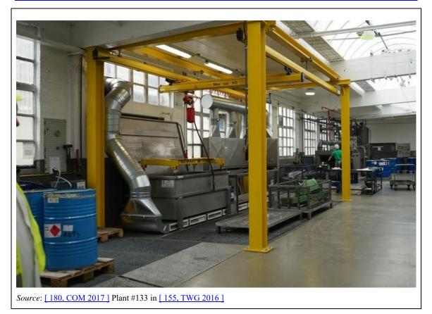
Figure 17.12:Enclosed automatic washing machine
