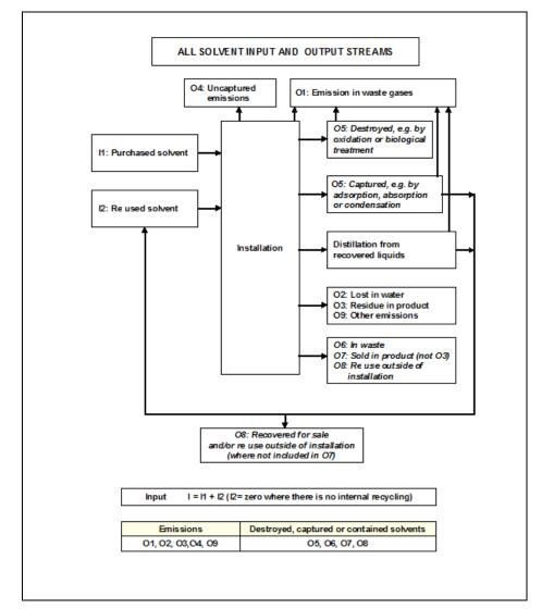
Figure 17.6: All solvent inputs and outputs (using definitions from the IED)
