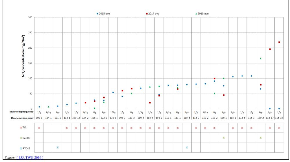
Figure 10.16: NO<sub>x</sub> emissions in waste gases for the period 2013-2015
