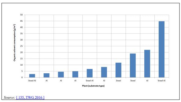
Figure 10.10:Organic solvent consumption from metal packaging installations (g of solvent input per m2 of product) - Average values for the period 2013-2015
