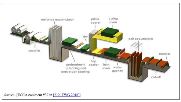
Figure 6.1: Typical layout of a coil coating line
