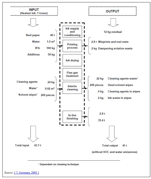
Figure 11.3: Specific input of substances and output of waste in a virtual heatset process
