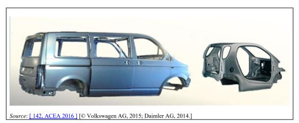
Figure 2.8: Examples of passenger car bodies showing the spread from very large to very small car bodies
