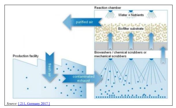
Figure 17.30: Scheme of the biological off-gas treatment system
