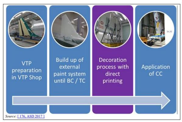
Figure 5.10: Process chain including direct printing
