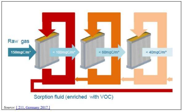
Figure 17.28: Filter cascade of absorption units
