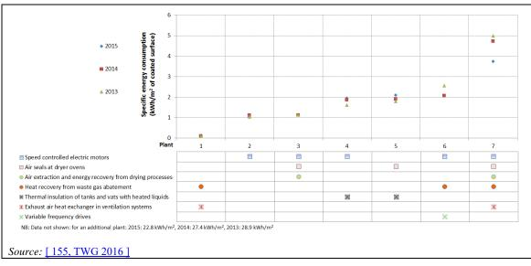
Figure 8.2: Specific energy consumption expressed in kWh per m<sup>2</sup> of coated surface for the period 2013-2015
