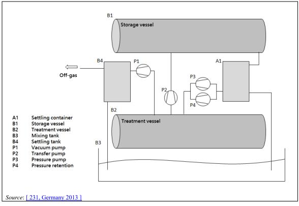
Figure 15.10: Example schematic of a pressure treatment plant for water-based preservatives
