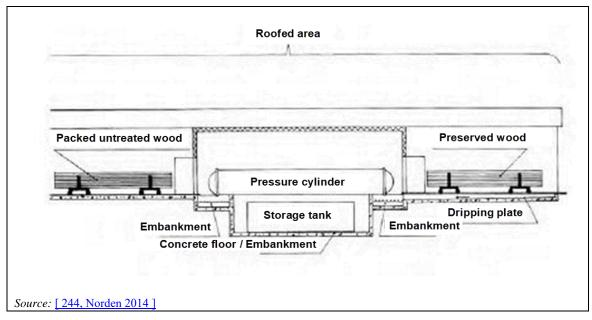
Figure 15.20:Schematic showing various options of precautionary measures (containment, drip pads, roof covers
