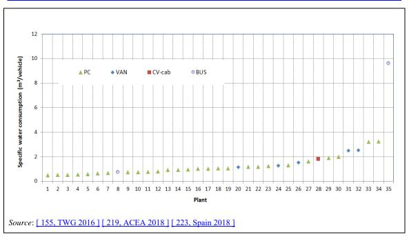
Figure 2.19: Specific water consumption (m<sup>3</sup>/vehicle) for automotive paint shops (2015 data)
