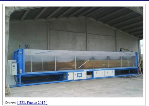
Figure 15.7: Wood in closed spraying tunnel
