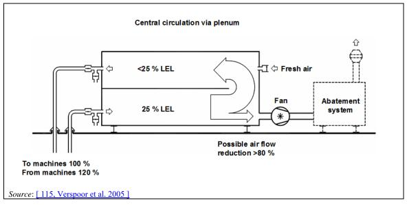
Figure 17.22: Plenum chamber
