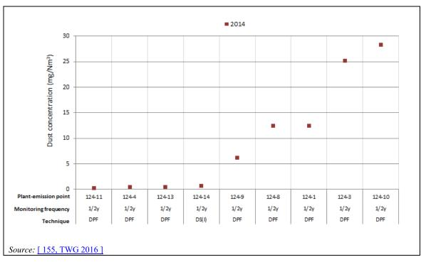
Figure 10.15: Dust emissions in waste gases (periodic monitoring) - Average values for the period 2013-2015
