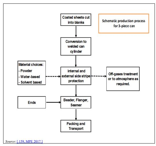
Figure 10.6: Production process for three-piece cans
