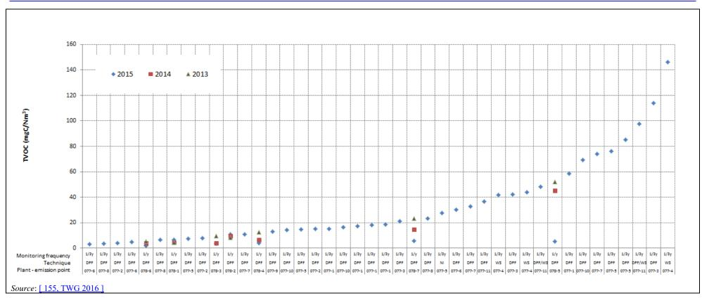
Figure 5.6: TVOC emissions in waste gases (periodic monitoring) - Average values for the period 2013-2015
