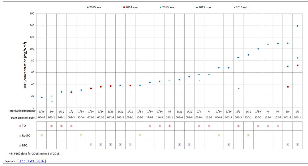
Figure 11.9: NO<sub>x</sub> emissions in waste gases for the period 2013-2015
