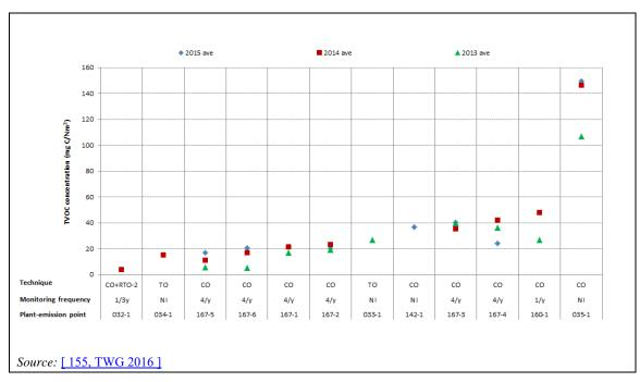
Figure 9.3: TVOC emissions in waste gases for the period 2013-2015
