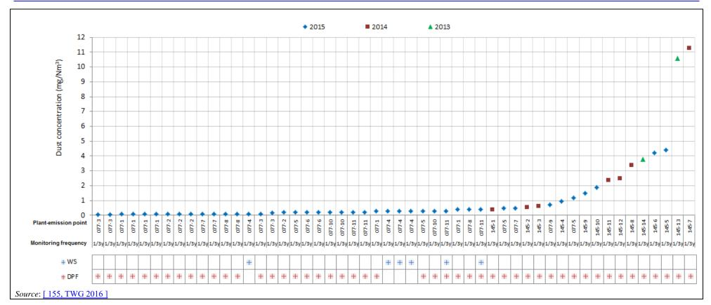
Figure 5.7: Dust emissions in waste gases (periodic monitoring) - Average values for the period 2013-2015
