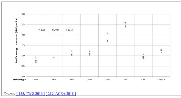
Figure 2.18: Specific energy consumption (MWh/vehicle) for van, truck and truck cabin coating plants
