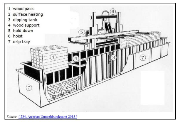
Figure 15.8: Schematic of trough impregnation
