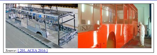
Figure 2.16: Coating operations for buses: e-coat (left) and topcoat (right)
