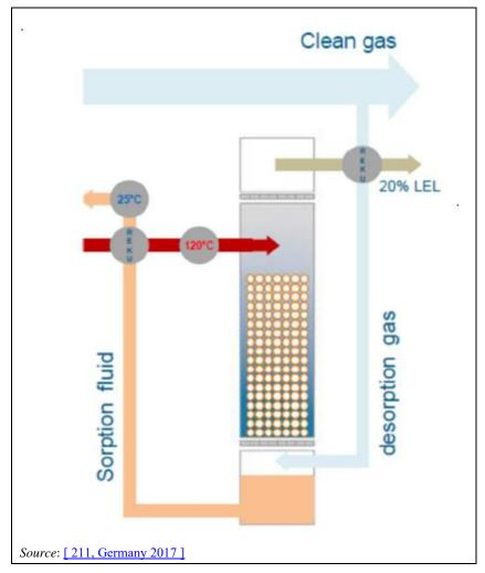
Figure 17.29: Characteristics of the desorption unit
