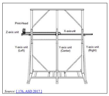
Figure 5.8: Gantry unit with all axes and printhead
