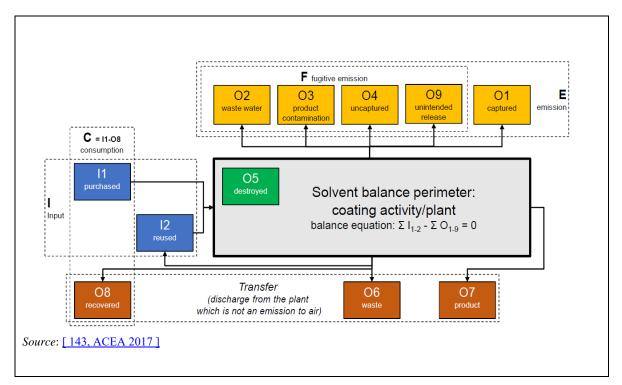
Figure 21.3: Solvent mass flows in a paint shop
