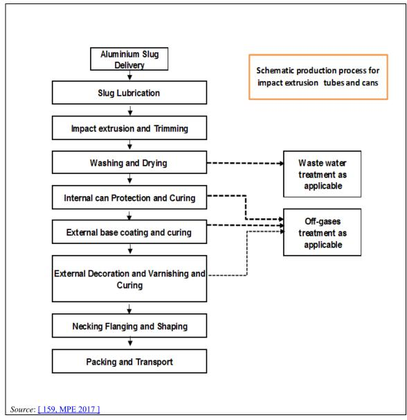
Figure 10.3: Production process of extruded aluminium tubes
