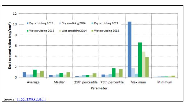
Figure 2.25: Statistical parameters of the reported dust emission data (periodic monitoring)
