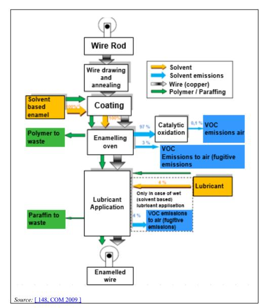
Figure 9.1: Typical manufacturing process and flow chart for winding wire manufacturing
