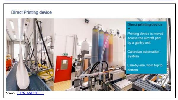
**Figure 5.13:** The direct printing device
