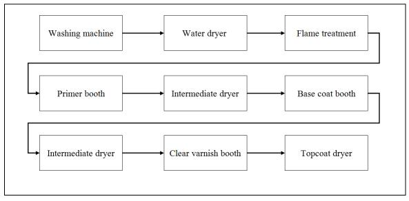
Figure 3.1: Water-based bumper coating process
