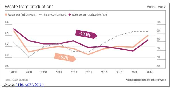
Figure 2.7: Waste generation from passenger car production (excluding scrap and demolition waste)
