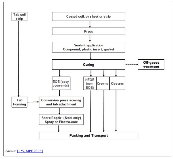
Figure 10.8: Production process for ends, crowns and closures
