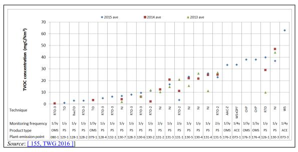
Figure 3.5: TVOC emissions in waste gases (periodic monitoring) - Average values for the period 2013-2015
