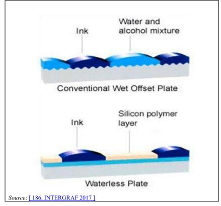
Figure 11.11: Conventional wet offset plate and waterless plate
