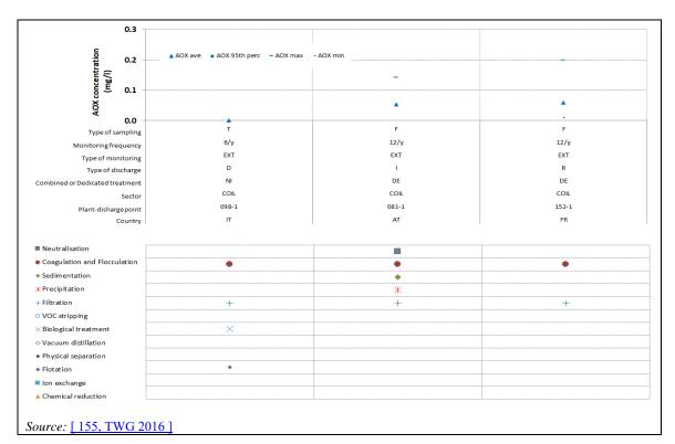
Figure 6.17: AOX concentration values for direct and indirect discharges of waste water from coil coating plants (data for 2015)
