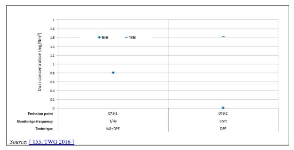
Figure 3.6: Dust emissions in waste gases (data for 2015)
