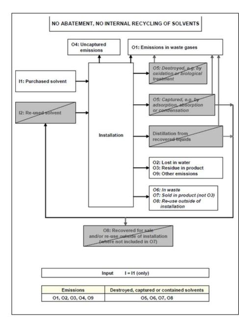
Figure 21.10: No end-of-pipe abatement and no internal recycling
