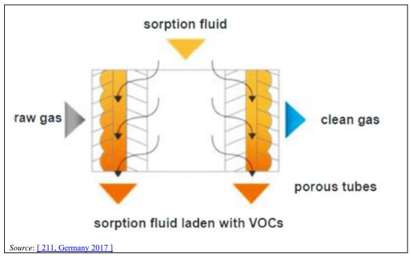
Figure 17.27: Keder tube in the absorption unit
