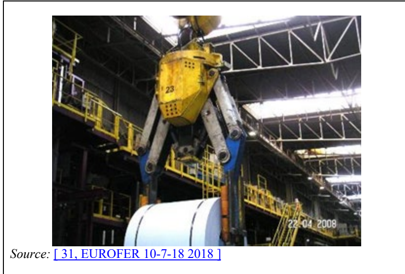
Figure 8.4: Coil tong with protector
