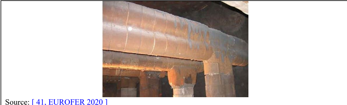
Figure 2.86: Double-pipes skid design for reheating furnaces
