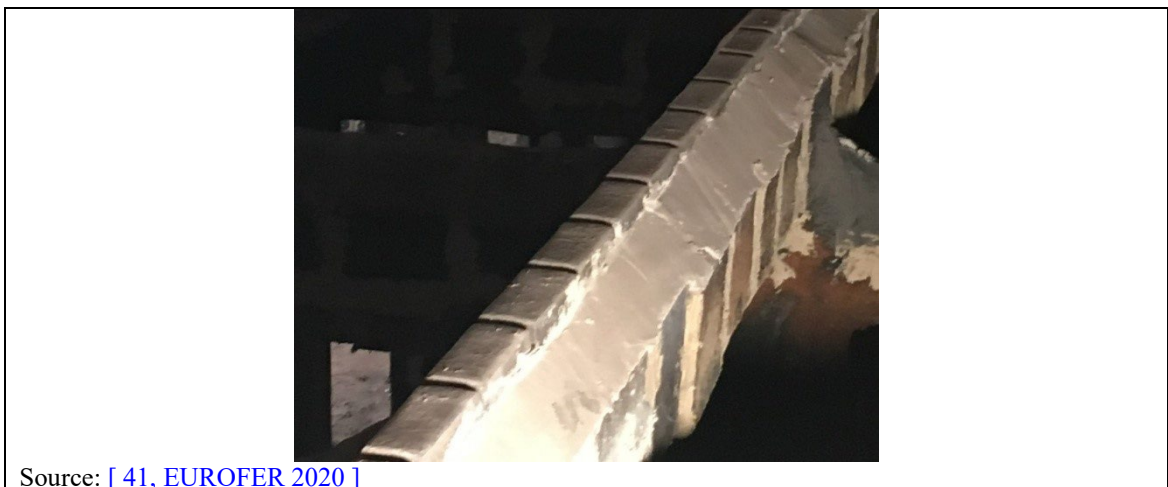
Figure 2.85: Skid riders design in a reheating furnace before hot rolling
