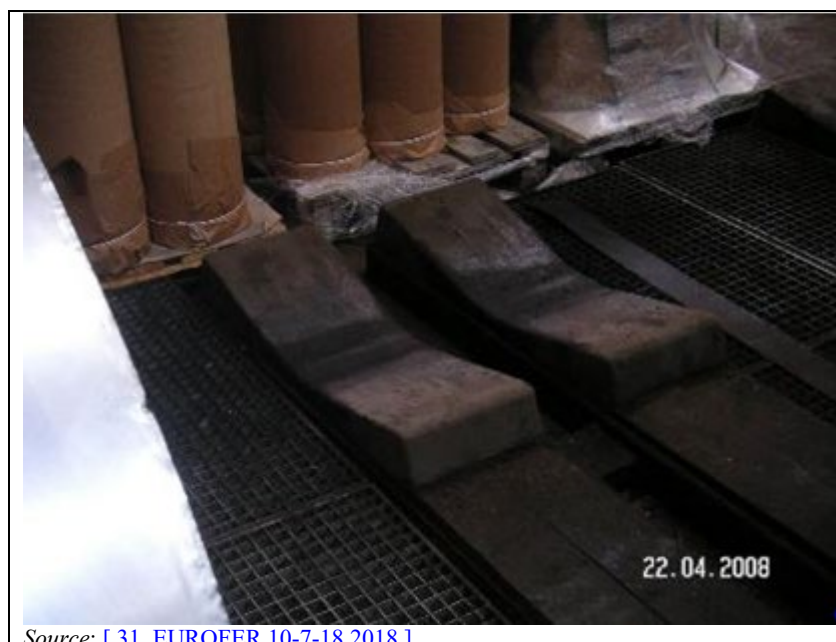
Figure 8.3: Coil support with oil drip trays
