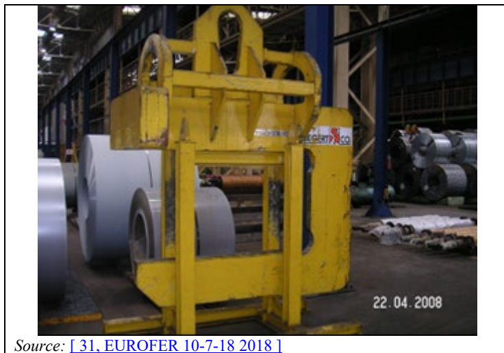
Figure 8.5: C-hook magnet for hoisting of coils
