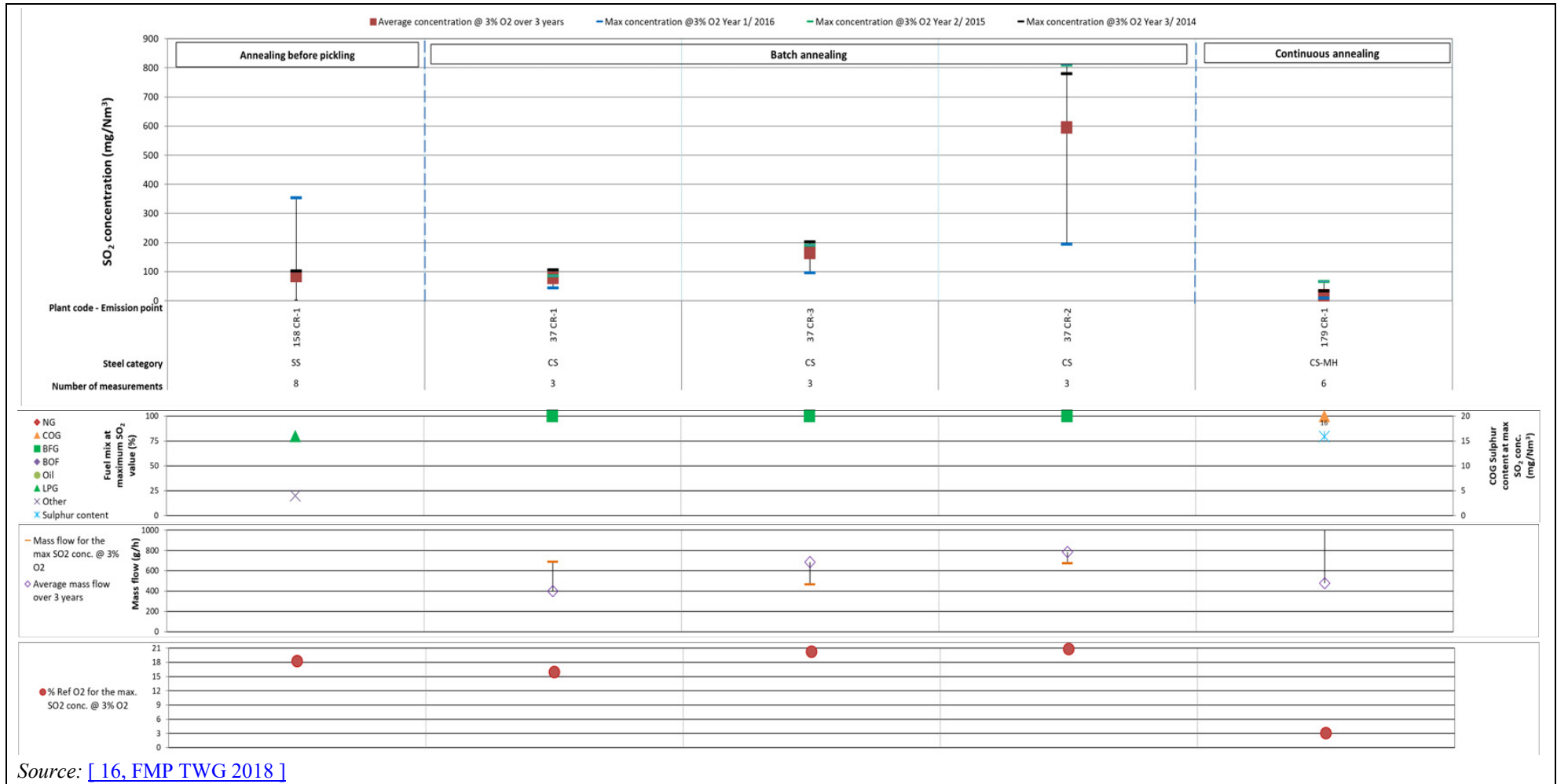
Figure 3.38: SO 2 emissions from feedstock heating (in mg/Nm 3 at 3 % oxygen) for fuels other than 100 % natural gas
