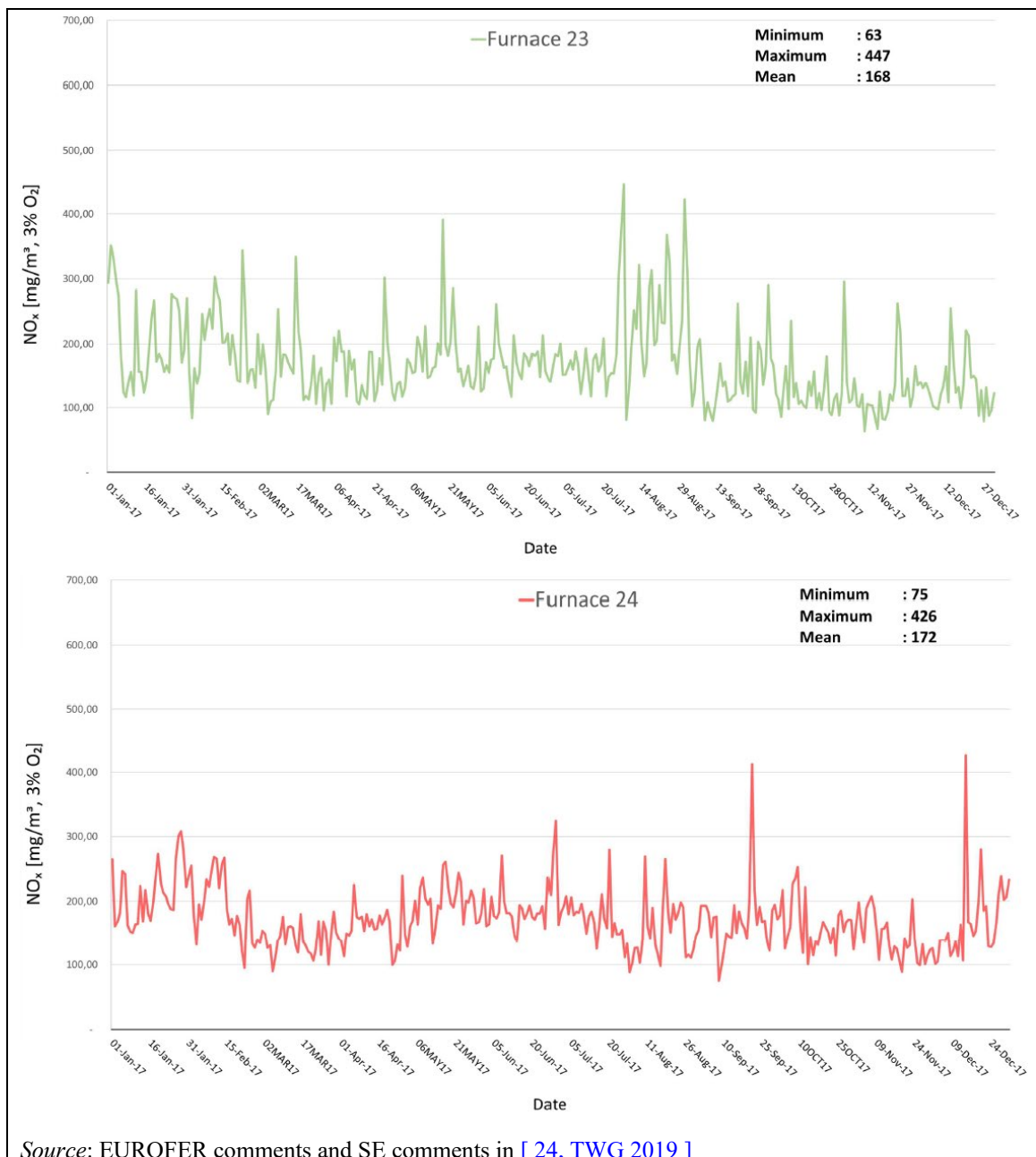
Figure 2.46: Continuously measured NO x emission concentrations at two walking beam furnaces from Tata Steel IJmuiden (Plant 110 HR2-2) showing NO x fluctuation over a year
