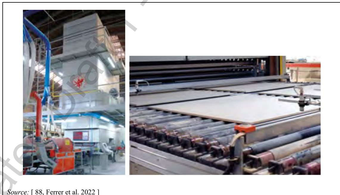
Figure 2-37: Vertical dryer for tiles
