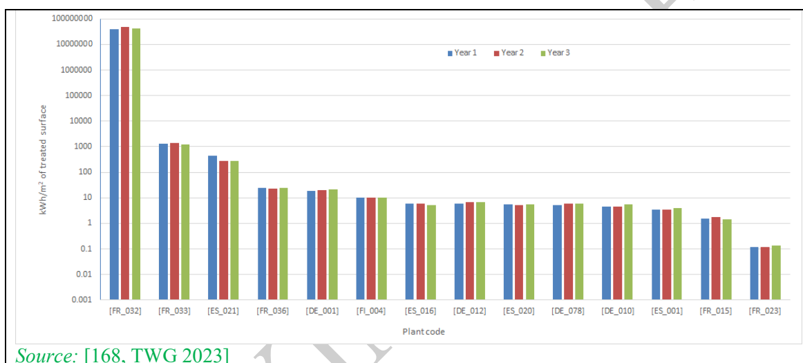
Figure 3-80: Specific energy consumption expressed in kWh per m 2 of treated surface in aluminium coil, sheet conversion coating and anodising plants
