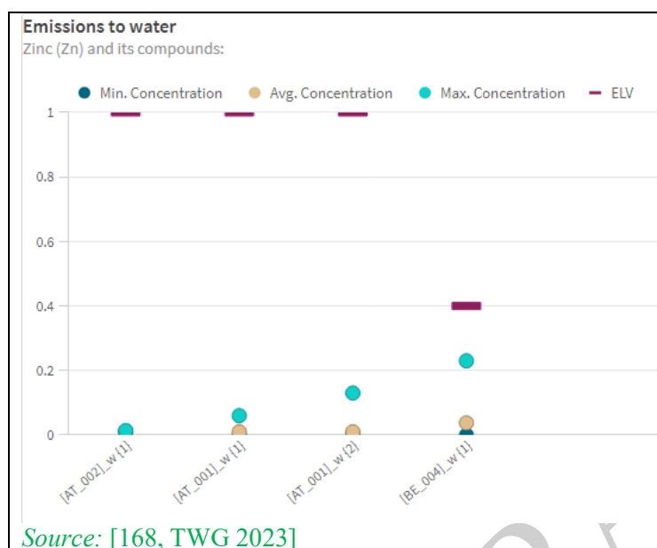
Figure 3-102: Zn emissions to water from PCB manufacturing plants
