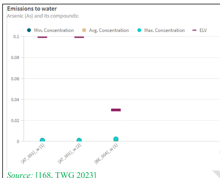
Figure 3-93: As emissions to water from PCB manufacturing plants
