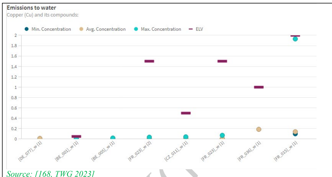
Figure 3-71: Cu emissions to water from aluminium coil, sheet conversion coating and anodising plants
