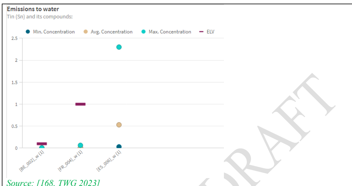
Figure 3-51: Sn emissions to water from continuous steel coil coating plants
