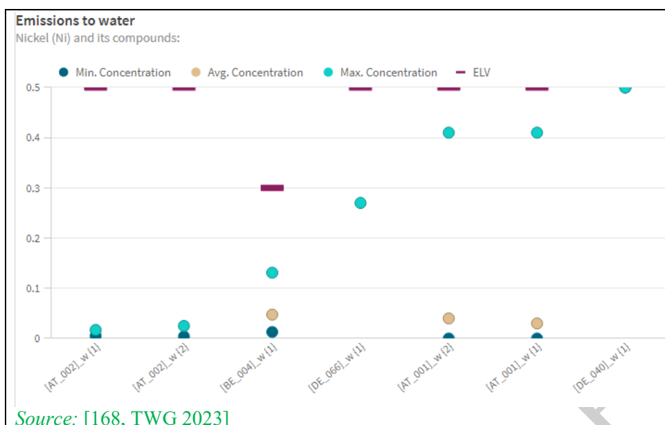
Figure 3-100: Ni emissions to water from PCB manufacturing plants
