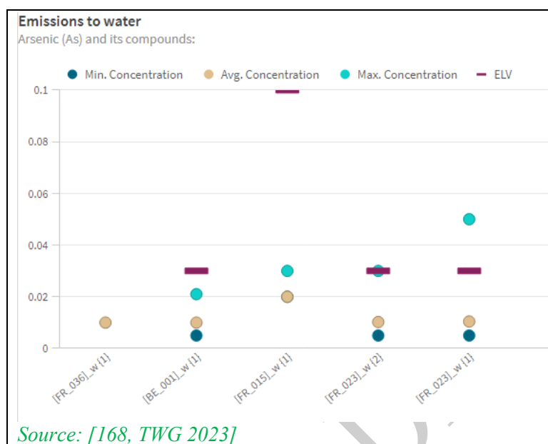
Figure 3-67: As emissions to water from aluminium coil, sheet conversion coating and anodising plants
