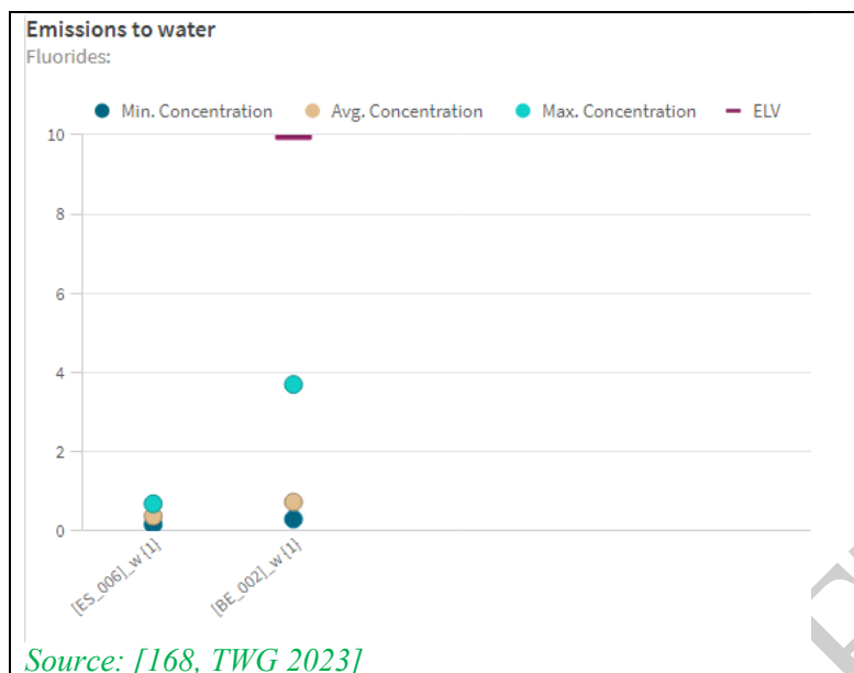
Figure 3-42: Fluorides emissions to water from continuous steel coil coating plants
