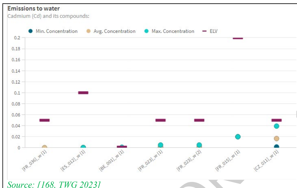
Figure 3-69: Cd emissions to water from aluminium coil, sheet conversion coating and anodising plants
