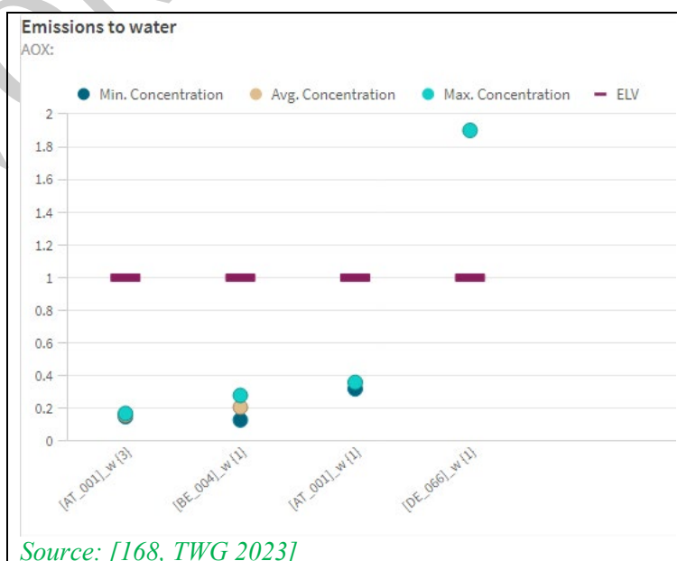
Figure 3-90: AOX emissions to water from PCB manufacturing plants
