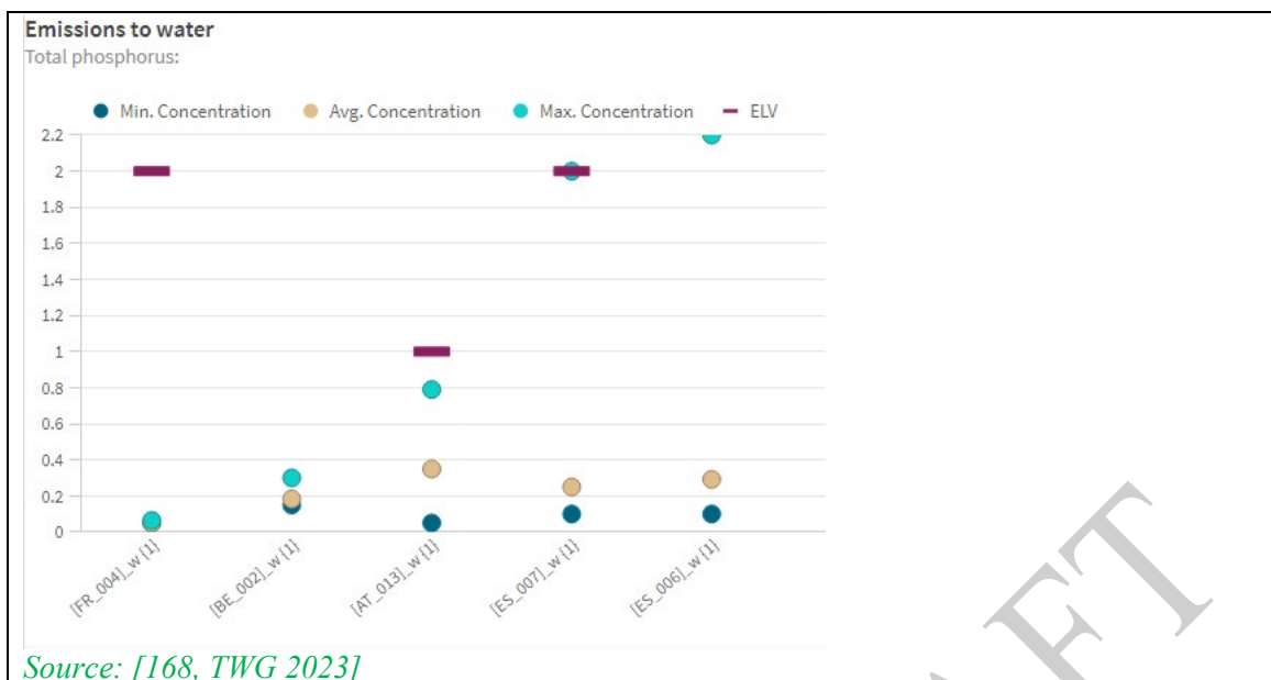
Figure 3-52: TP emissions to water from continuous steel coil coating plants
