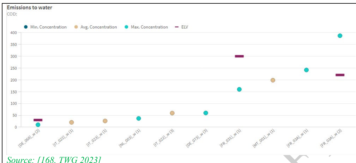
Figure 3-110: COD emissions to water from semiconductor manufacturing plants
