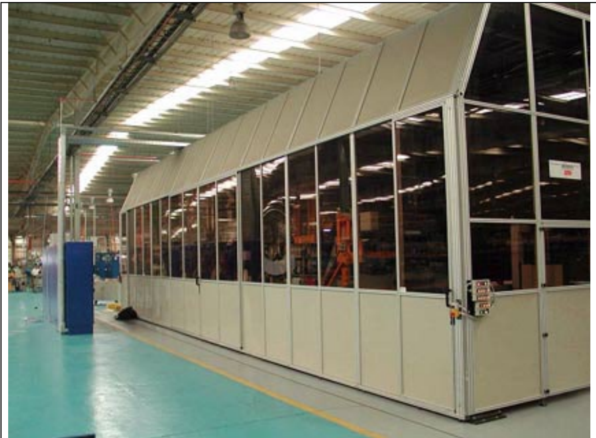
Figure 4-6: Encapsulated integrated chromium plating line
