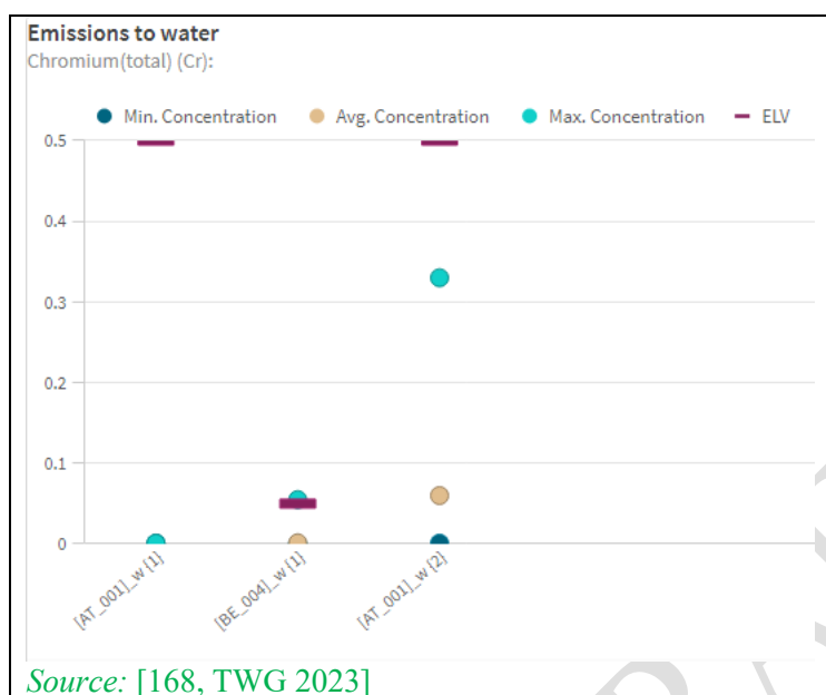
Figure 3-97: Cr emissions to water from PCB manufacturing plants
