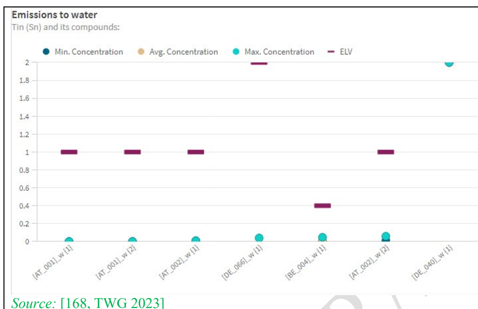
Figure 3-101: Sn emissions to water from PCB manufacturing plants
