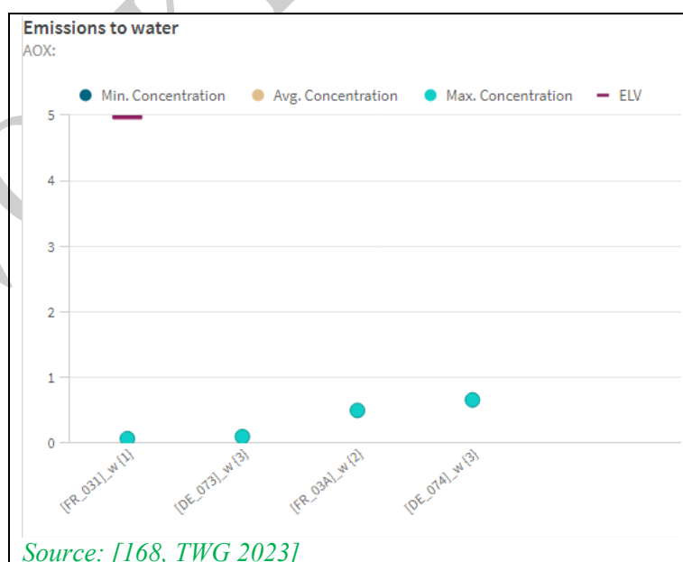
Figure 3-113: AOX emissions to water from semiconductor manufacturing plants
