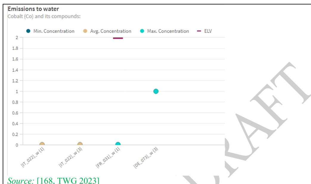
Figure 3-120: Cobalt emissions to water from semiconductor manufacturing plants
